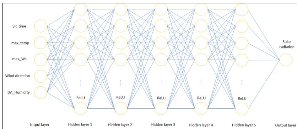
Figure 4. The general structure of the proposed DNN.
