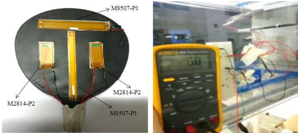
Figure 6. Positions of piezoelectric materials on the membrane wing and current measurements
