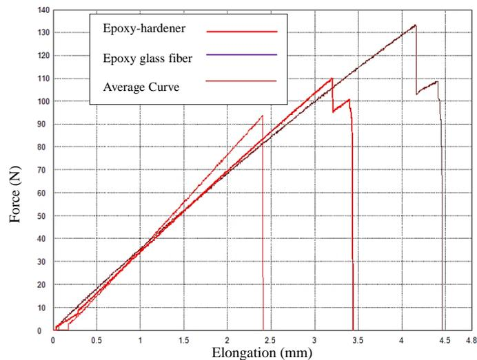
**Figure 12.** Bending force-elongation graph of the epoxy-hardener
