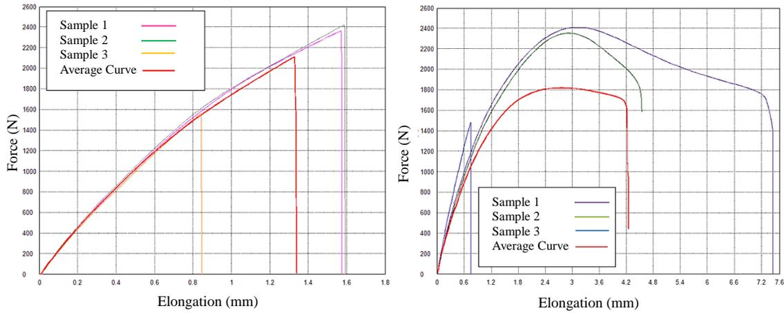
**Figure 10.** Tensile force-elongation graph of graphene epoxy nanocomposite a) 0.4 mg/mL b) 0.8 mg/mL
