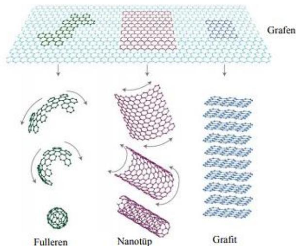
**Figure 4.** Carbon-based materials [21]
