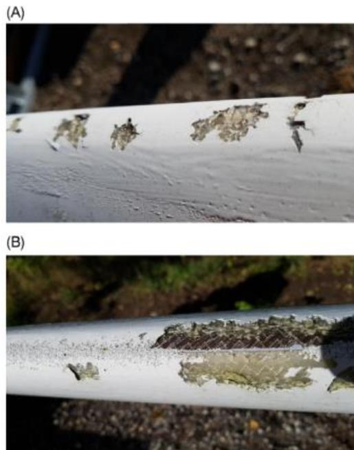
**Figure 2.** Leading-edge of a wind turbine blade with erosion A) initiation case, B) developed stage [10]
