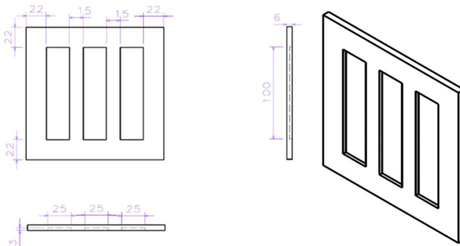
Figure 6. Sketch of the mold for the desired specimen (length units were mm)
