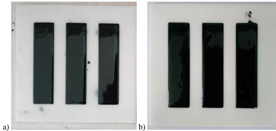
**Figure 7.** Graphene epoxy nanocomposite prepared with glass fiber in the amount of 0.4 mg/mL, b) graphene epoxy nanocomposite prepared with glass fiber in the amount of 0.8 mg/mL
