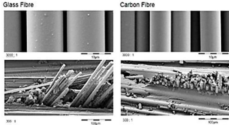
**Figure 3.** Enlarged view of glass and carbon fibers in free and composite structure [19]
