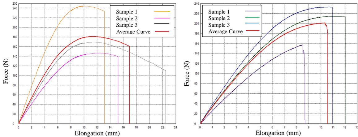
Figure 14. Bending force-elongation graph of the graphene epoxy with glass fiber a) 0.4 mg/mL b) 0.8 mg/mL
