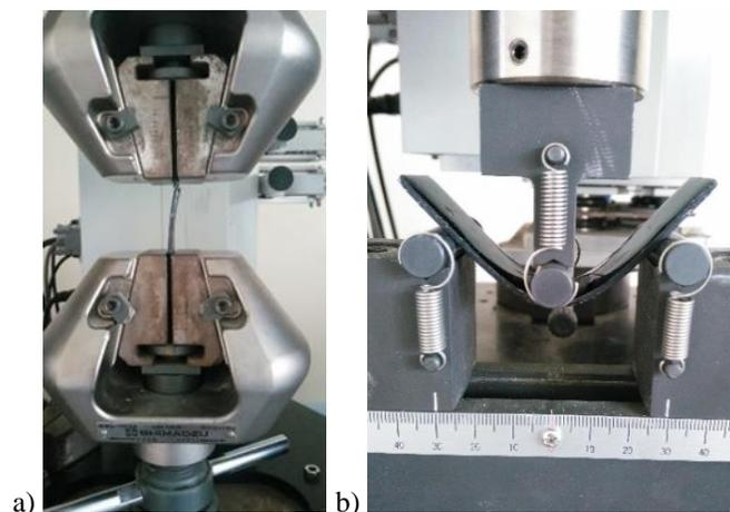
**Figure 8.** Tests for the prepared specimens in a) Tensile testing, b) Three-point bending testing
