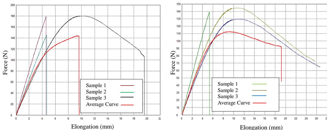
**Figure 13.** Bending force-elongation graph of the graphene epoxy nanocomposite a) 0.4 mg/mL b) 0.8 mg/mL
