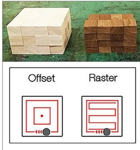
**Figure 1.** Untreated and thermo-treated ash wood samples for machining in two strategies: *offset* and *raster*
