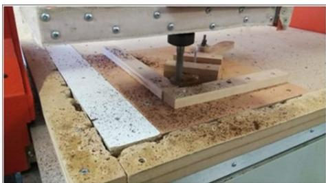
**Figure 3.** CNC machine (BDARK 2120 PRO, Turkey) in face milling operation
