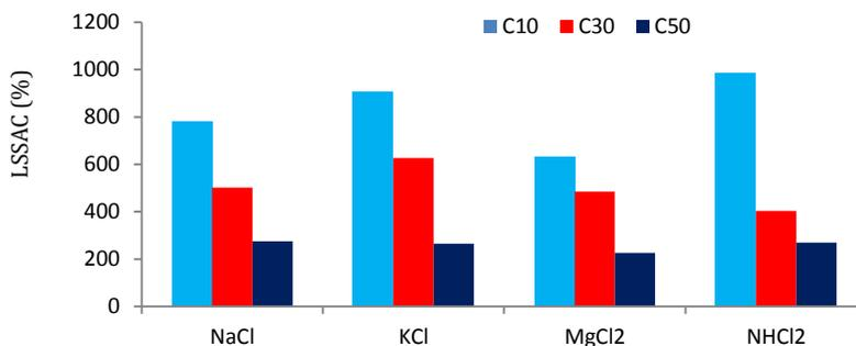
**Figure 2.** Liquid absorption capacity and swelling values of cellulosic SAP control samples in different salt solutions
