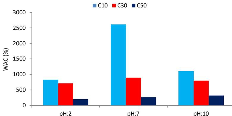
**Figure 1.** Water Absorption Capacity of Cel-SAPs which were prepared Dissolving pulp cellulose and CMC mixture with citric acid crosslinking method
