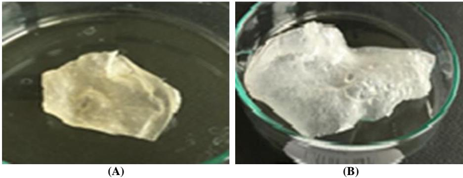
**Figure 3.** Photos of cellulosic superabsorbent. (A) Dry sheet form, (B) After water uptake.
