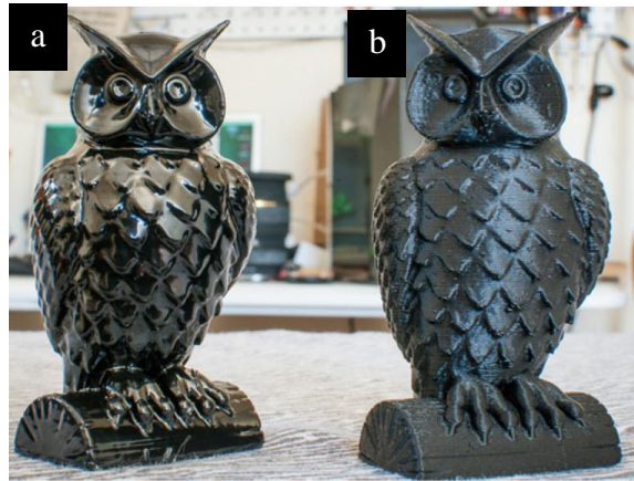
Figure 10. (a) Acetone vapour smoothed ABS parts. (b) As-built [43].
