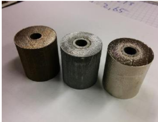
Figure 6. LAM manufactured test pieces. On the left without coating, middle chromium coated and right bright nickel coated [28] .
