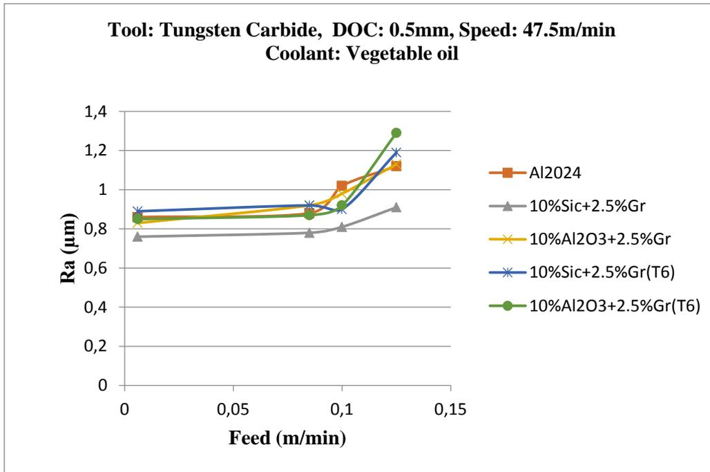
**Figure 10.** Surface roughness using Tungsten carbide tool with feed rate at 47.5 m/min speed
