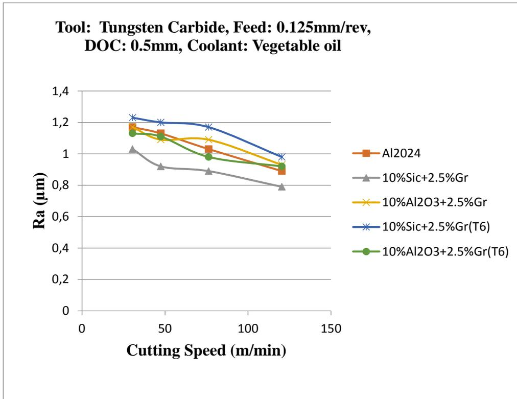
**Figure 8.** Surface roughness using Tungsten carbide tool with depth of cut at feed 0.125 mm/rev
