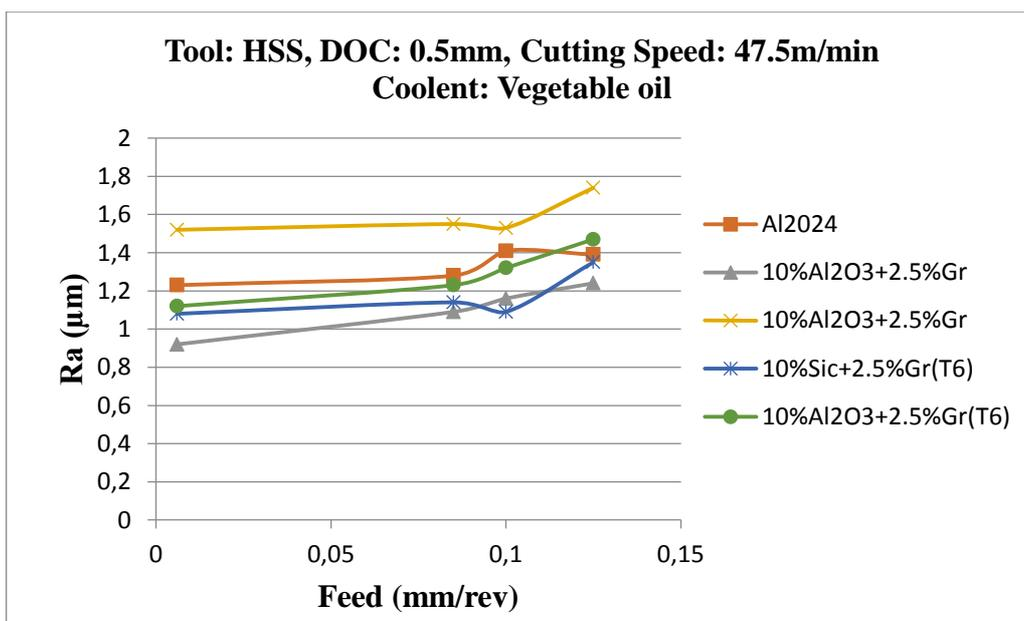
**Figure 9.** Surface roughness using HSS tool with feed rate at 47.5 m/min speed
