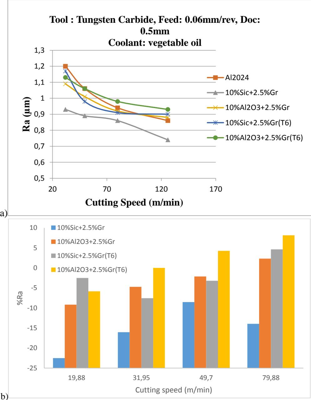
**Figure 4.** Surface roughness using Tungsten carbide tool with cutting speed a) Surface roughness with respect to Al2024, b) %Change in surface roughness
