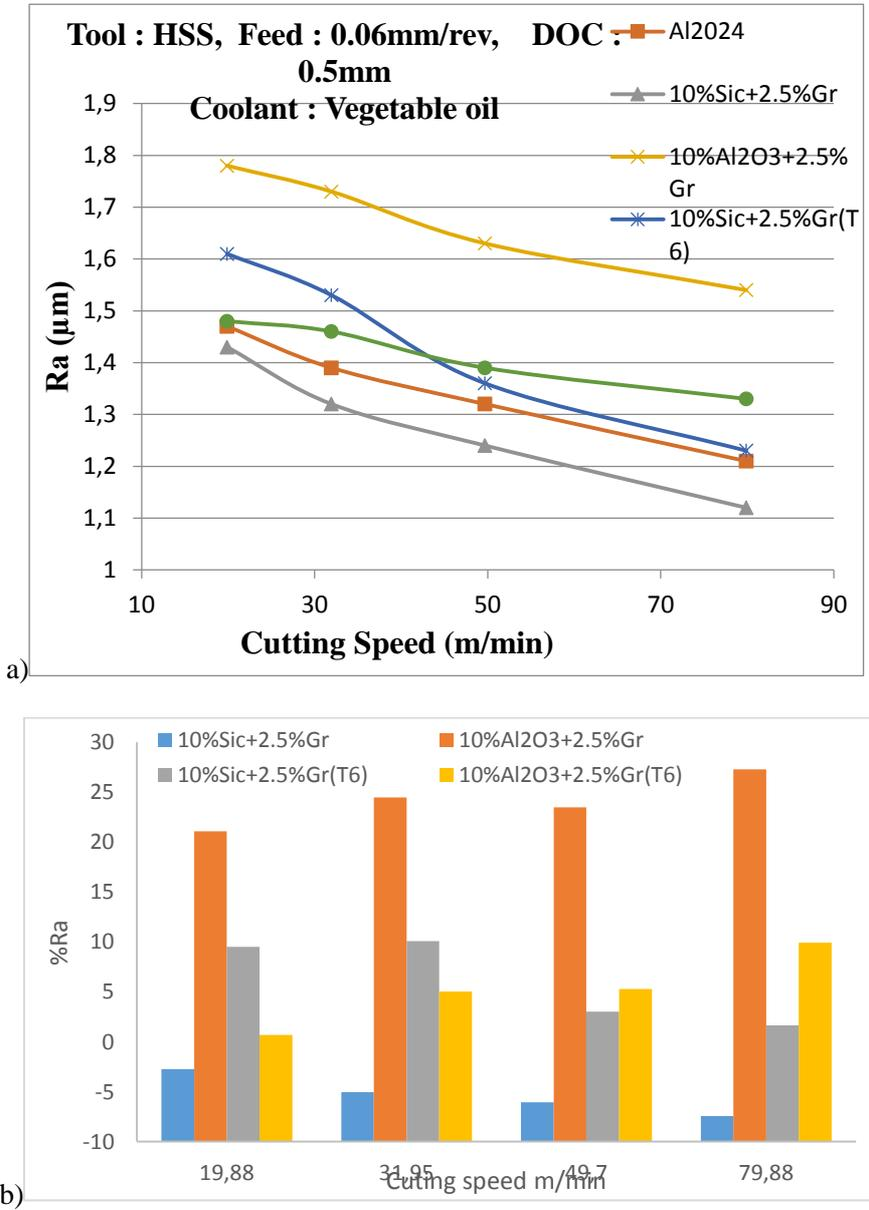
**Figure 3.** Surface roughness using HSS tool with cutting speed a) Surface roughness with respect to Al2024, b) % change in surface roughness
