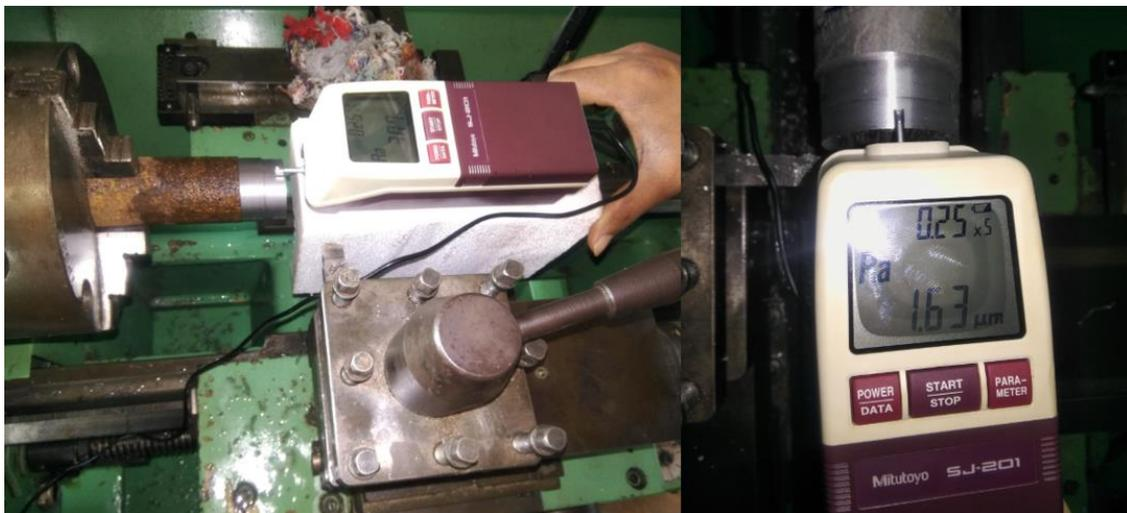
**Figure 2.** Surface roughness measurement on the work piece
