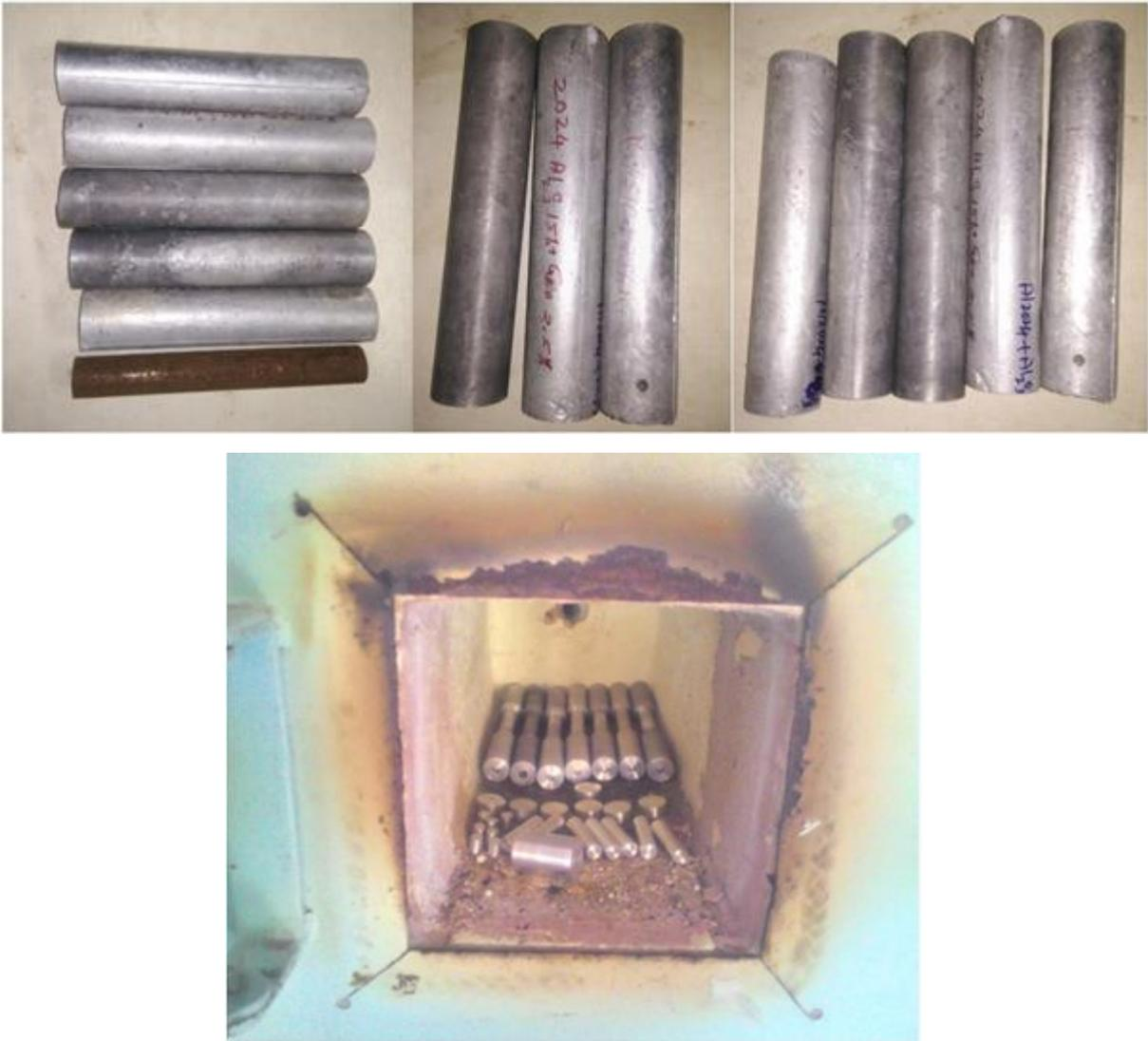
**Figure 1.** Composite rods and heat treatment of material for hardening
