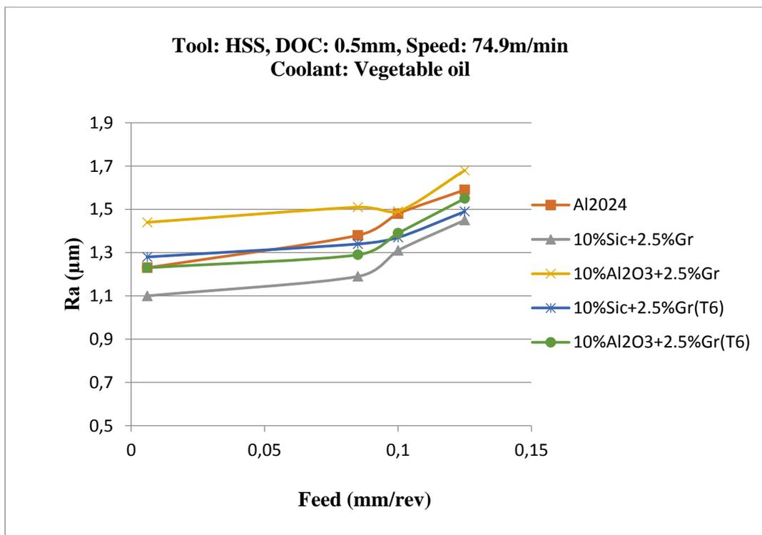
**Figure 11.** Surface roughness using HSS tool with feed rate at 74.9 m/min speed
