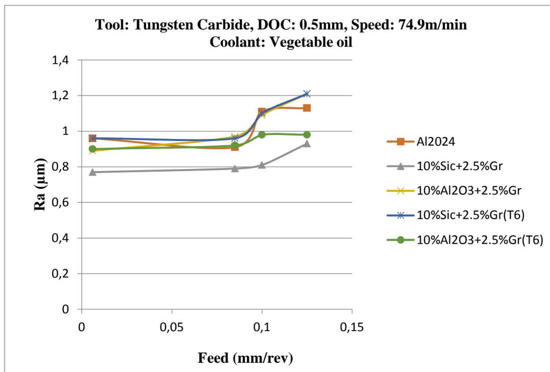
**Figure 12.** Surface roughness using Tungsten carbide tool with feed rate at 74.9 m/min speed
