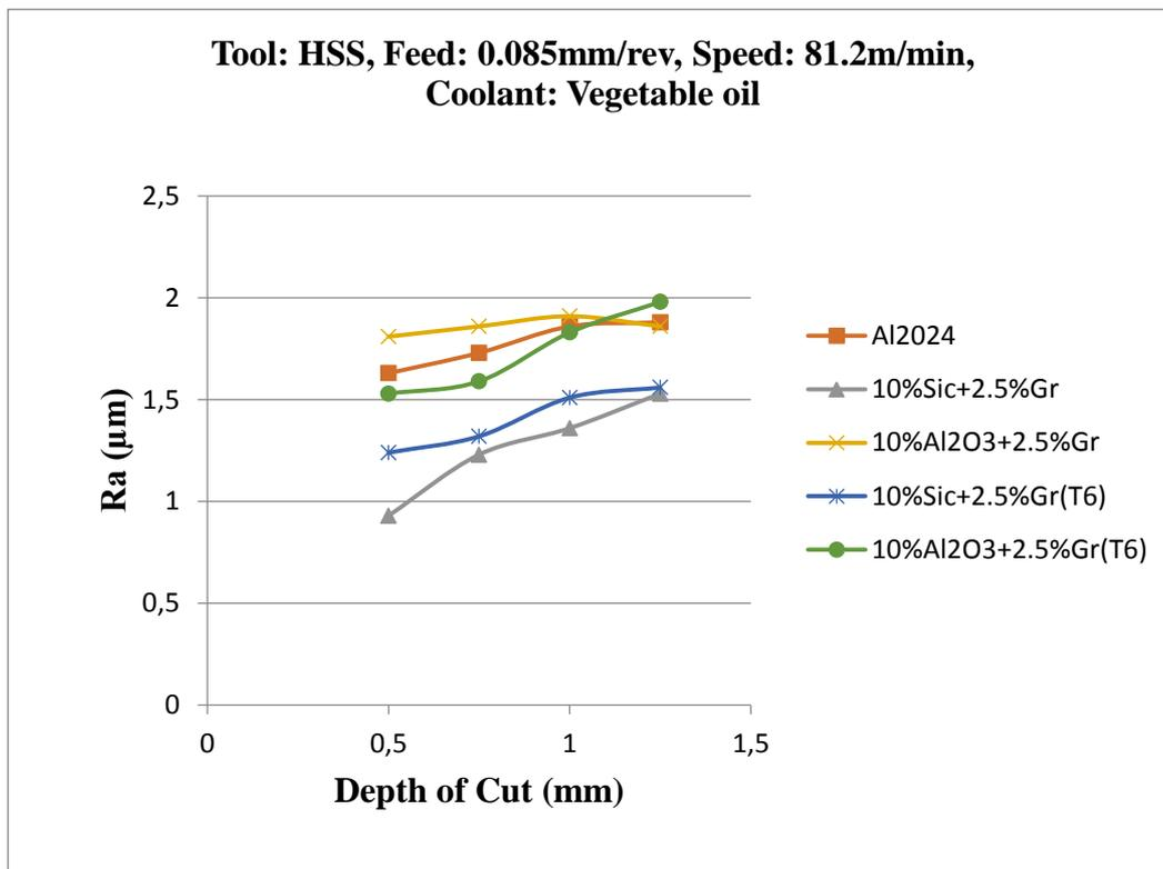
**Figure 5.** Surface roughness using HSS tool with depth of cut at feed 0.085 mm/rev
