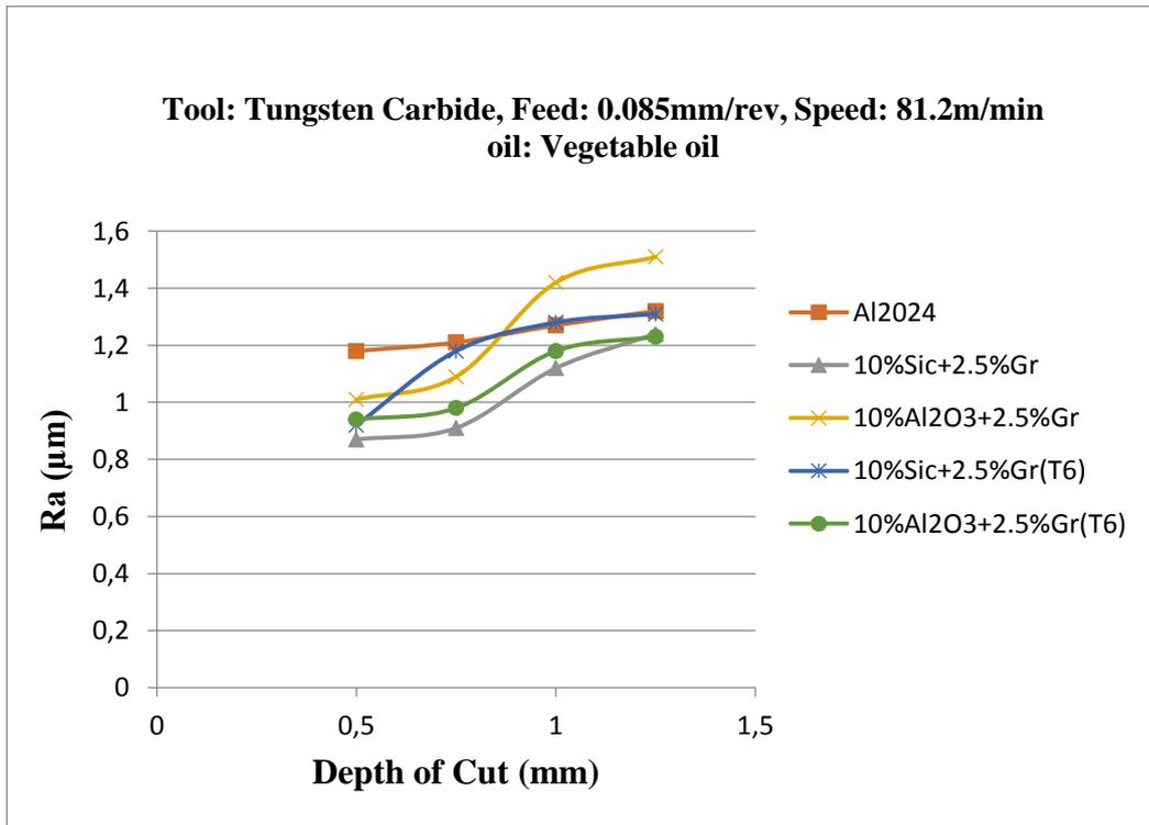
**Figure 7.** Surface roughness using Tungsten carbide tool with depth of cut at feed 0.085 mm/rev
