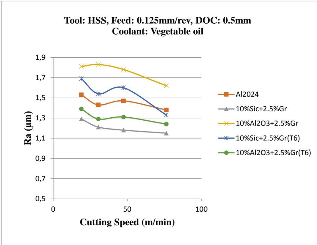
**Figure 6.** Surface roughness using HSS tool with cutting speed at feed 0.125 mm/rev
