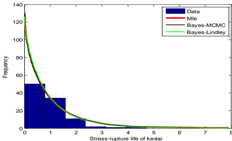
**Figure 6.** The histogram and fitted densities for stress-rupture life of kevlar data
