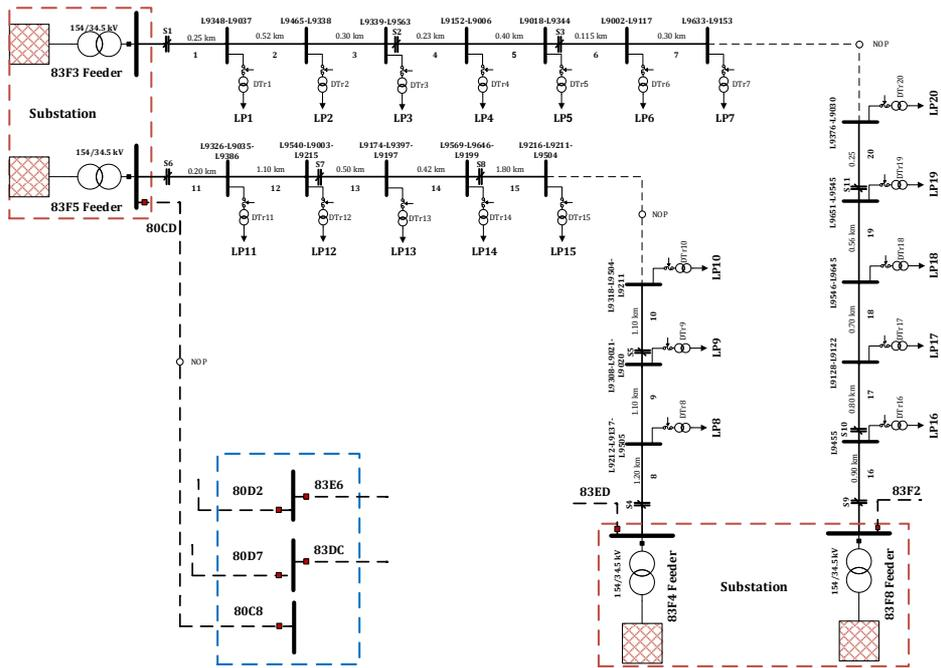
Figure 2. Single line diagram of BEDAS 4-Feeders distribution system
