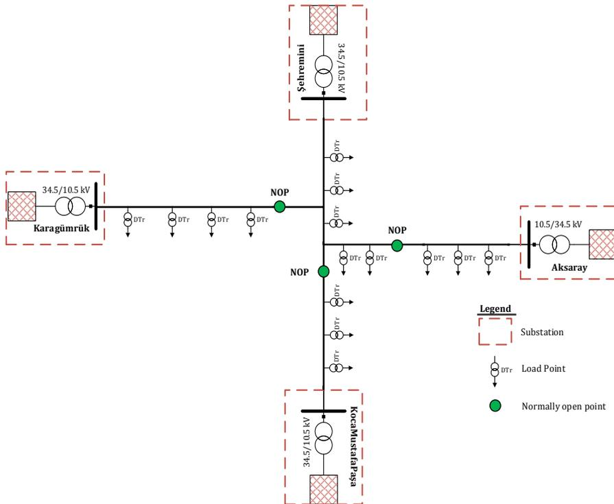
Figure 1. Bayazit-Beyoglu distribution section mes hed designed radial-operated
