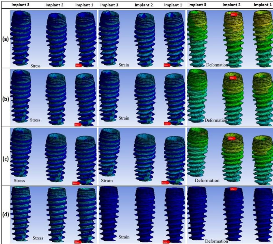
**Figure 7.** Stress, strain and deformation in the dental implant: (a)CoCr, (b)Zr, (c)Ti, (d)PEEK.
