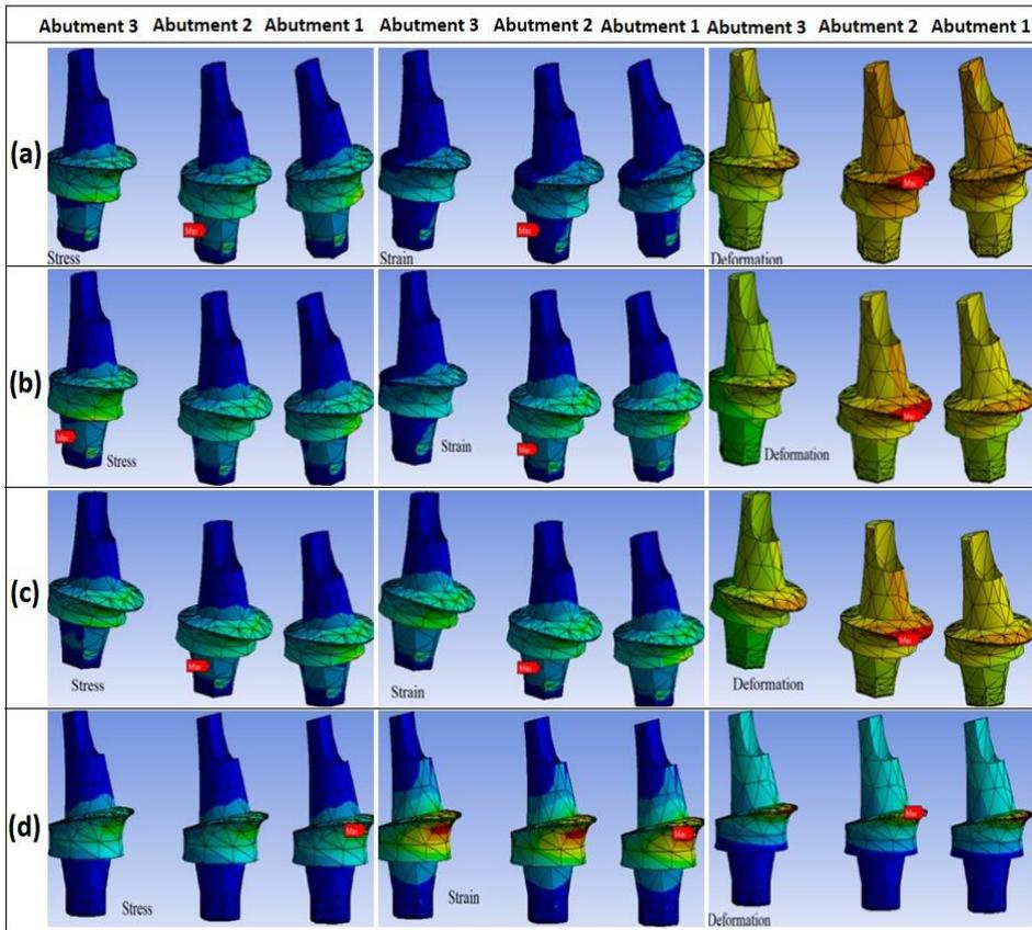
**Figure 8.** Stress, strain and deformation in the abutment: (a)CoCr, (b)Zr, (c)Ti, (d)PEEK.
