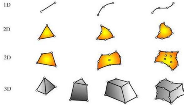
**Figure 1.** Finite element types (one-dimensional, two-dimensional and three-dimensional)
