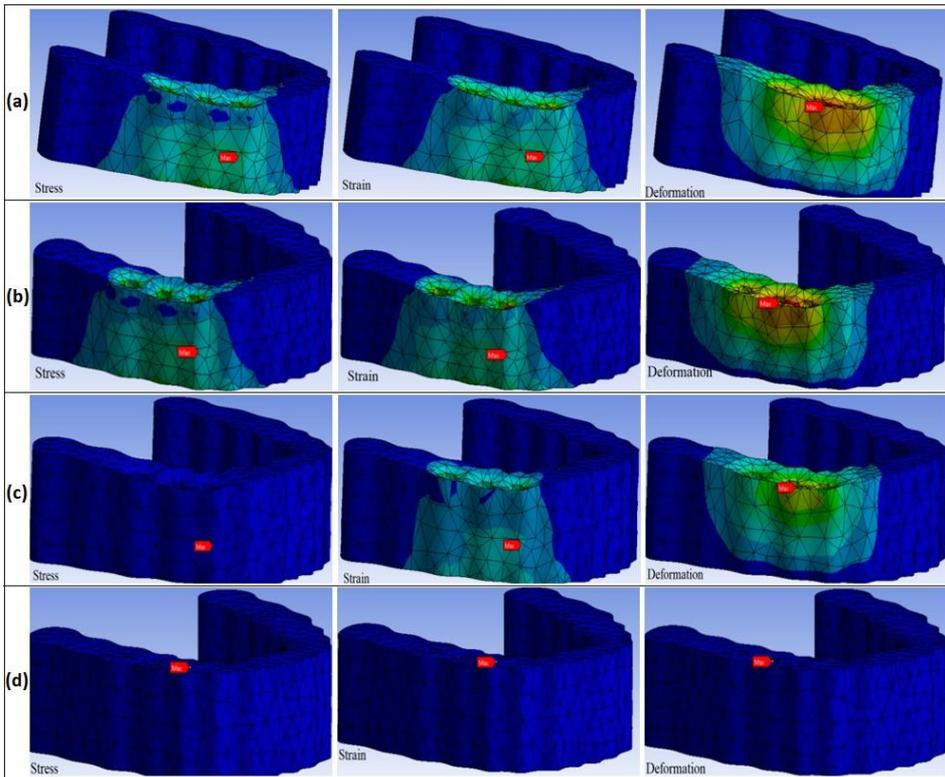
**Figure 6.** Analysis images of the stress, strain and deformation in the bone when using; a) CoCr, b) Zr, c) Ti and d) PEEK as the abutment material.
