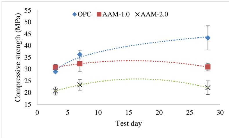
Figure 7. Compressive strength results
