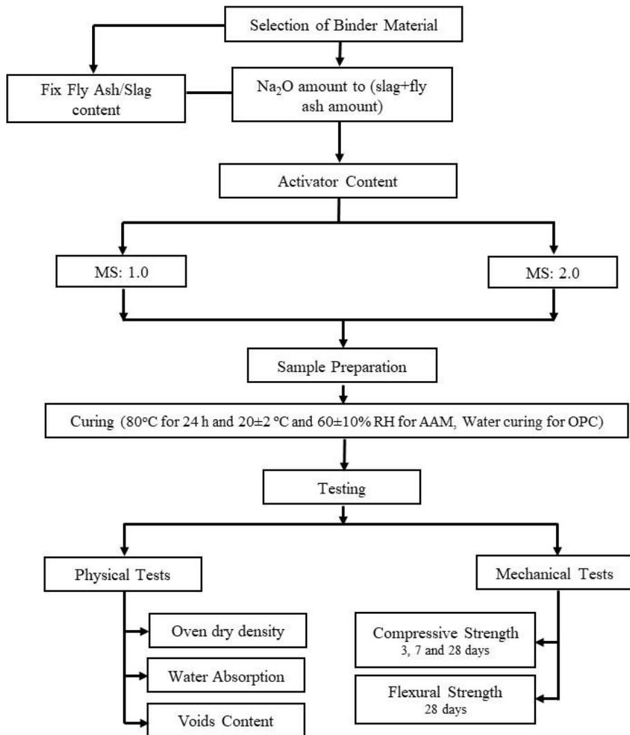
**Figure 2.** Flow chart of the experimental study
