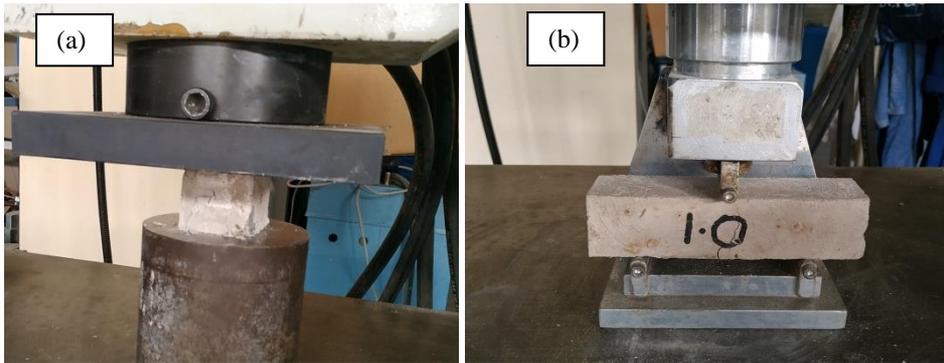
**Figure 3.** Mechanical testing of samples (a) compressive strength test (b) flexural strength test
