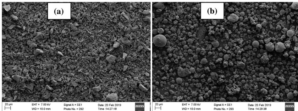
**Figure 1.** SEM micrographs of (a) GGBS and (b) FA
