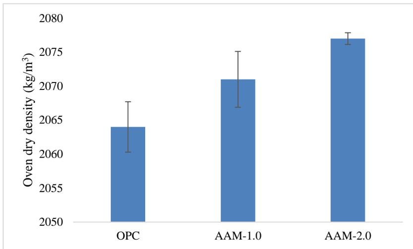
**Figure 4.** Dry density results of the mixes
