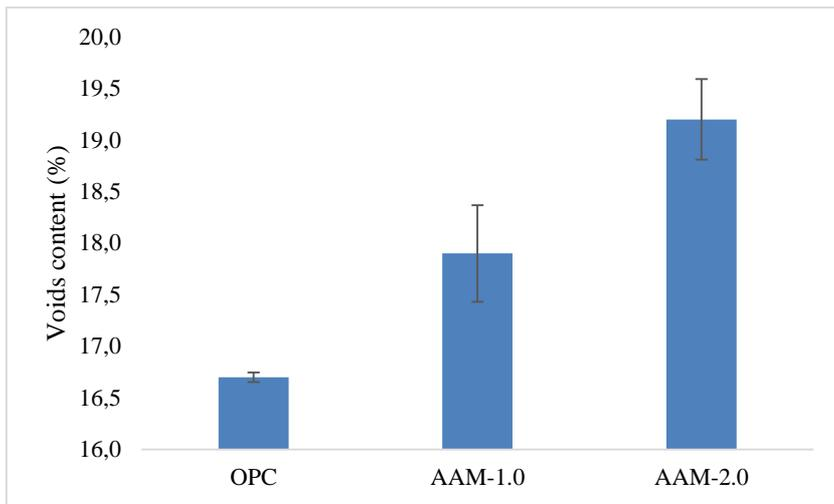
**Figure 6.** Voids content results of the mixes
