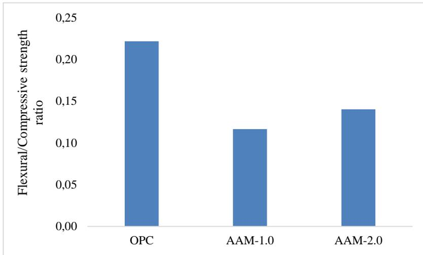
**Figure 9.** Comparison of flexural/compressive strength ratio of the mixes
