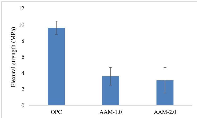
Figure 8. Flexural strength results
