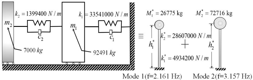
**Figure 4.** Input and output parameters obtained for modal analysis
