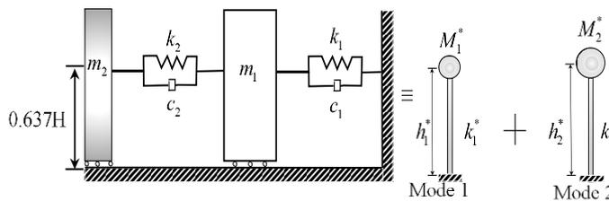
**Figure 2.** Mathematical model of wall-backfill system considered
