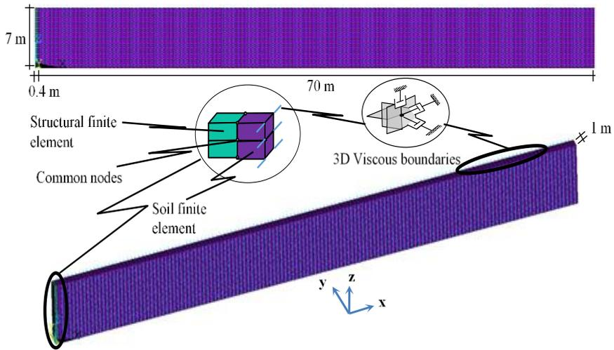
**Figure 3.** Schematic representation of the finite element model under fixed base
