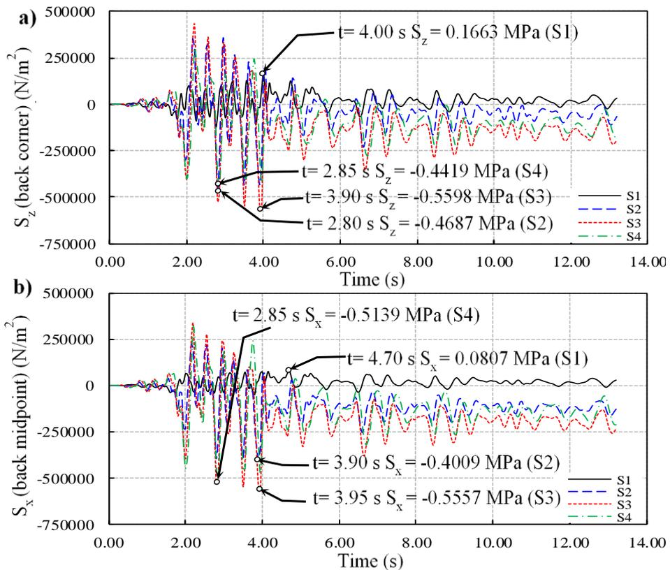
**Figure 8.** The peak stress-time history obtained from a) back corner of the wall in z direction b) back midpoint of the wall in x direction
