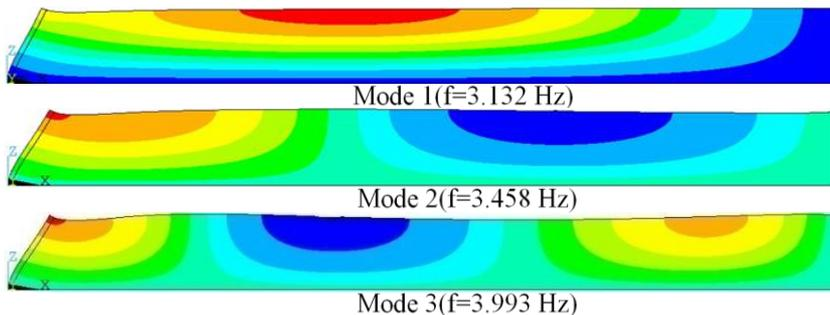
**Figure 5.** Mode frequencies and mode shapes obtained from FEM
