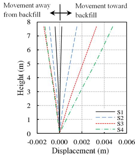
**Figure 9.** The relative horizontal displacement obtained along the cantilever wall height
