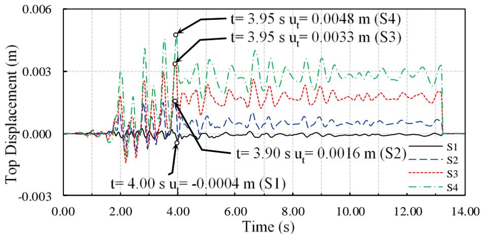
**Figure 10.** Time history of the horizontal top displacement of the cantilever retaining wall
