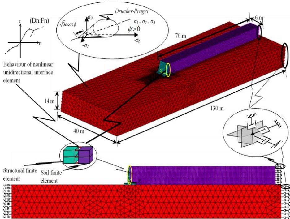
**Figure 6.** Schematic representation of the soil structure interaction system
