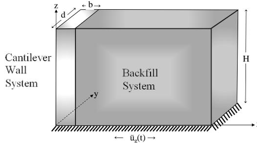
**Figure 1.** Wall-backfill system considered for mathematical model
