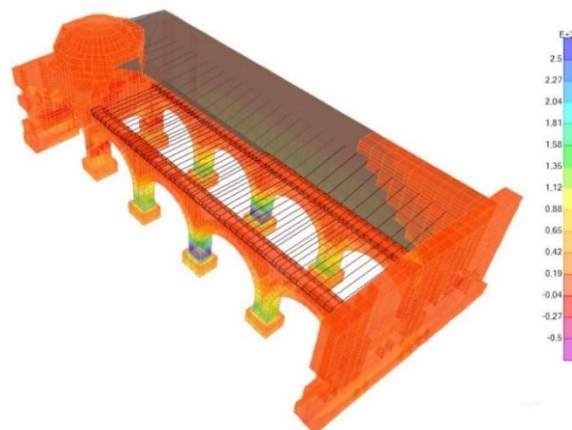
Figure 11. Maximum S33 tensile stresses of the mosque subject to Düzce earthquake
