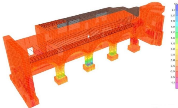
Figure 9. Maximum S33 tensile stresses of the mosque subject to Erzincan earthquake
