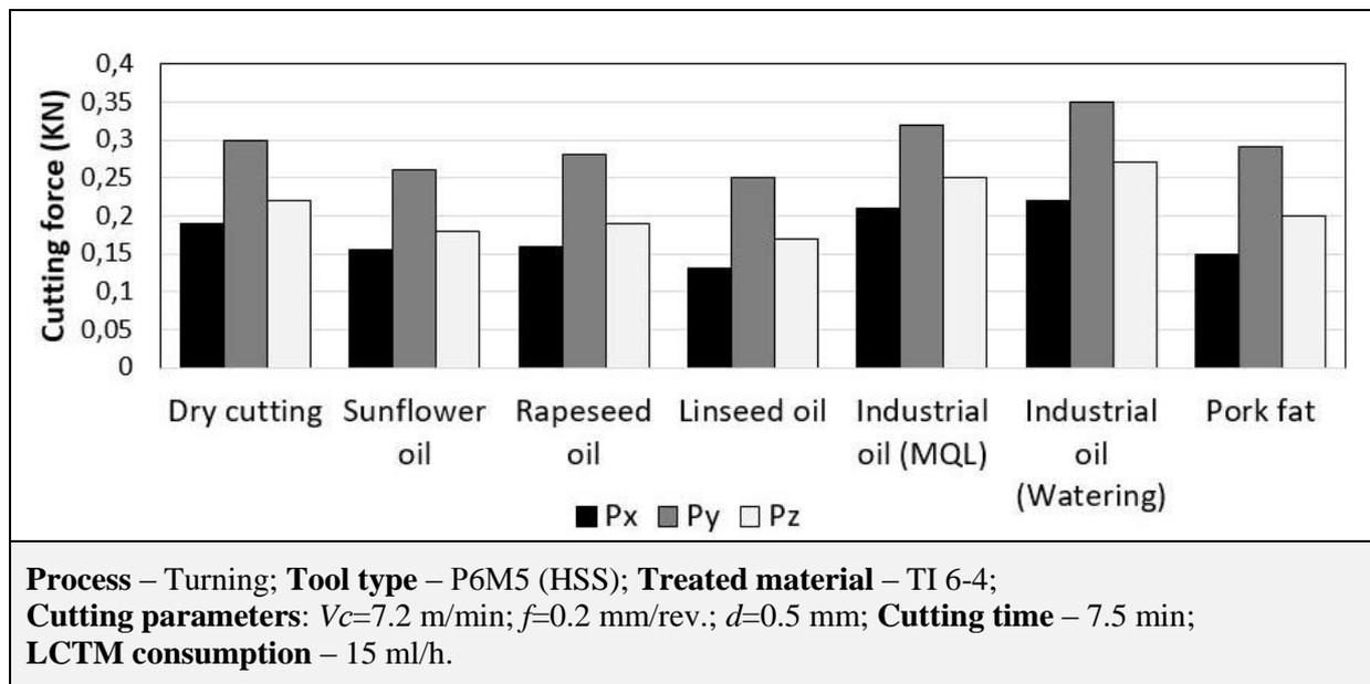
**Figure 6.** Effect of vegetable and animal oils on the cutting force in the processing of titanium alloy TI 6-4
