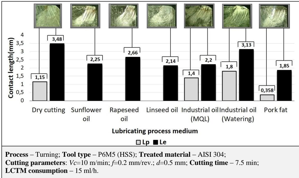
**Figure 7.** Effect of oils of plant and animal origin on the length of plastic and elastic contact (Lp and Le) when processing stainless steel AISI 304
