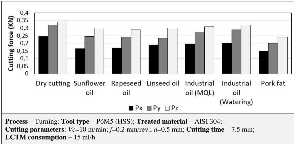
**Figure 5.** Effect of vegetable and animal oils on the cutting force in the processing of stainless steel AISI 304
