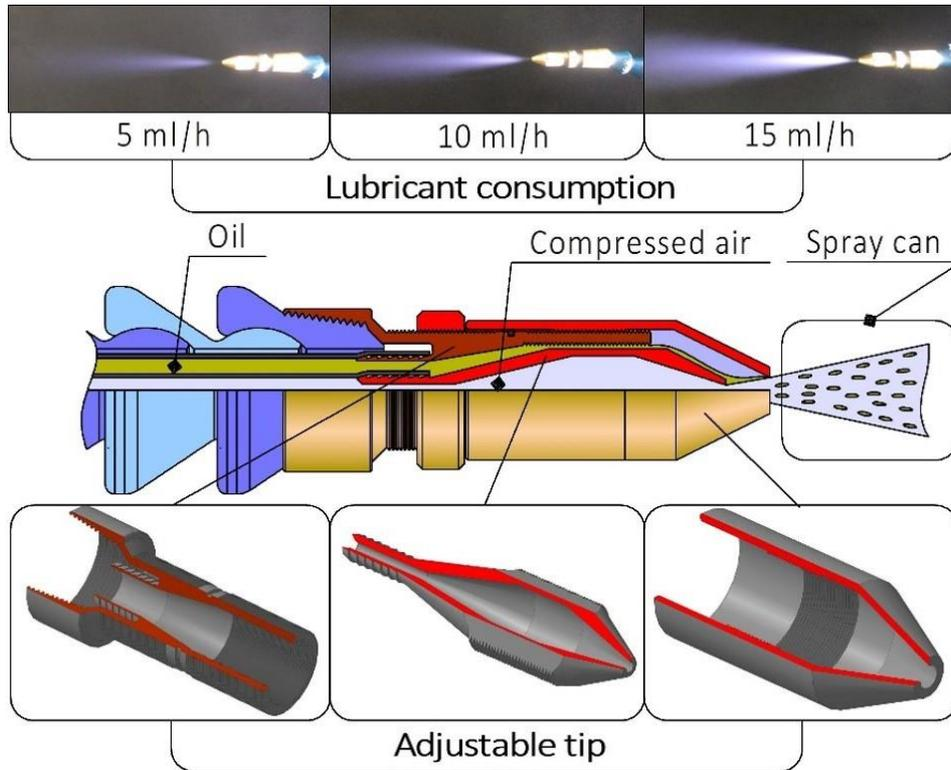
**Figure 1.** General view of the MQL dosing device
