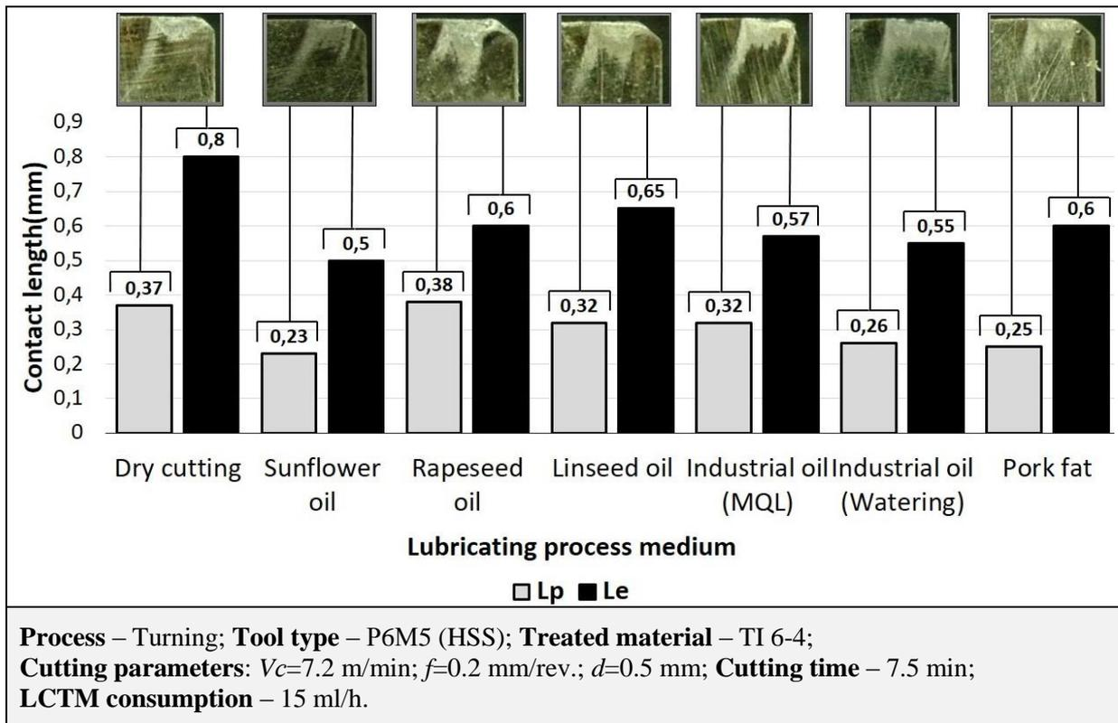
**Figure 8.** Effect of oils of plant and animal origin on the length of plastic and elastic contact (Lp and Le) when processing titanium alloy TI 6-4
