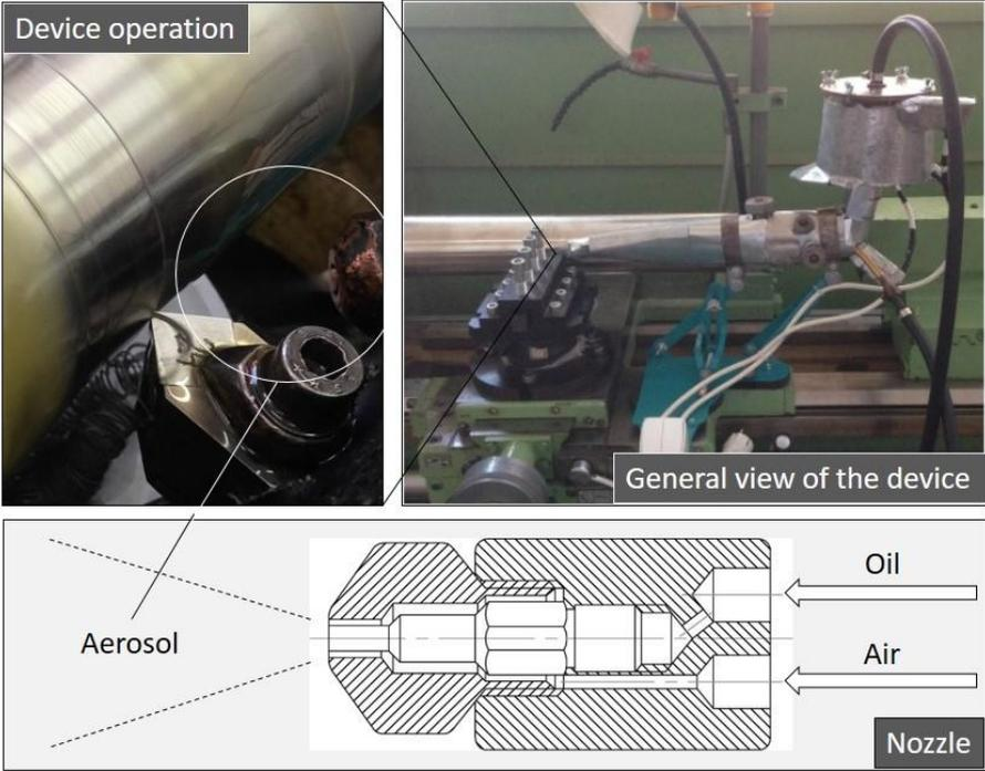
**Figure 3.** General view of the metering device for spraying animal fats into the cutting zone
