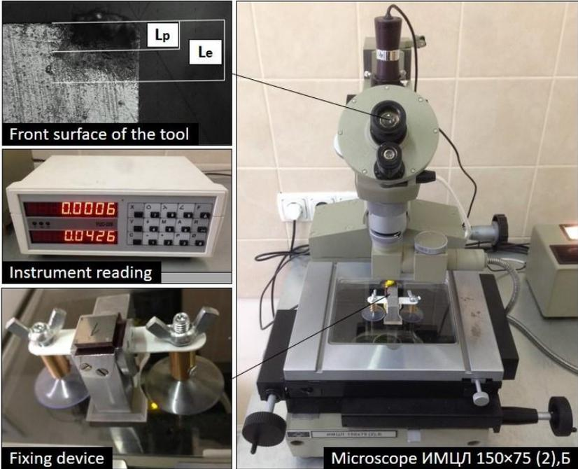
**Figure 4.** Measurement of zones of plastic and elastic contact ( $L_p$  and  $L_e$ )
