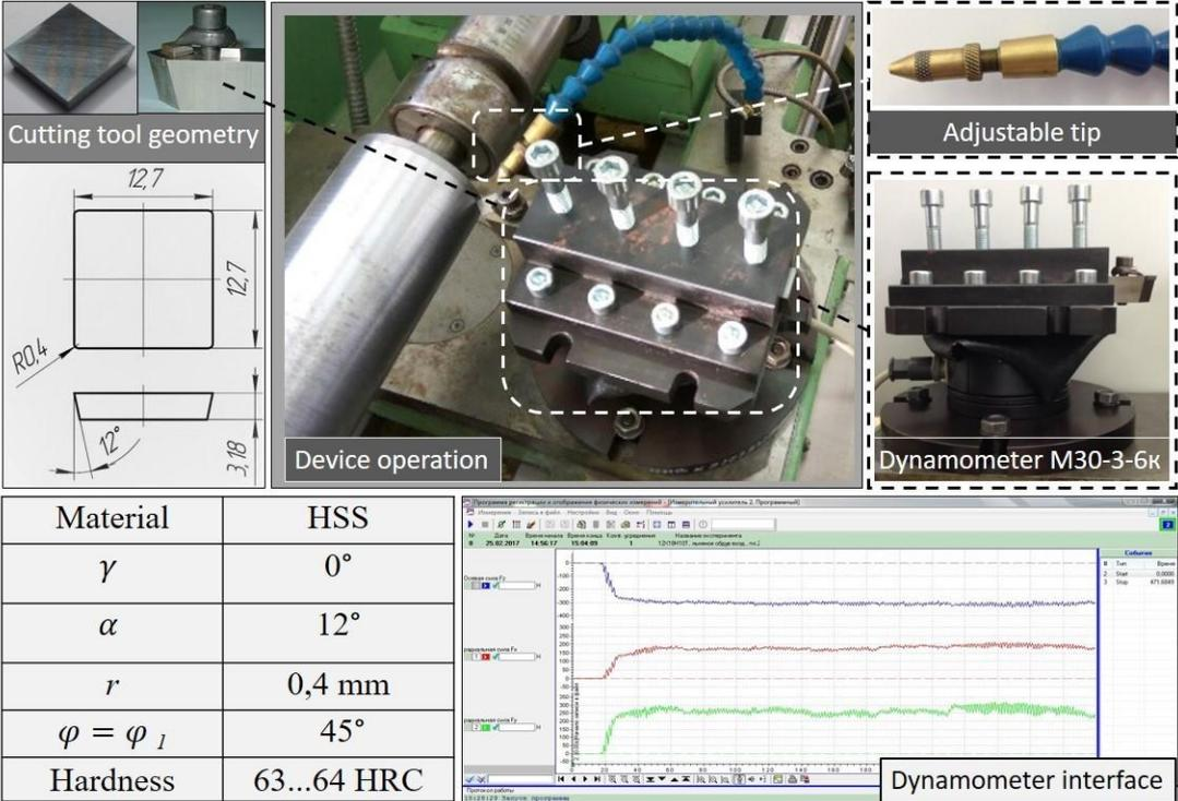
**Figure 1.** Geometrical parameters of the cutting tool. Three-component dynamometer (M-30-3-6k)
