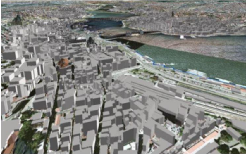
Figure 8. Part of the 3D city model in LoD1
