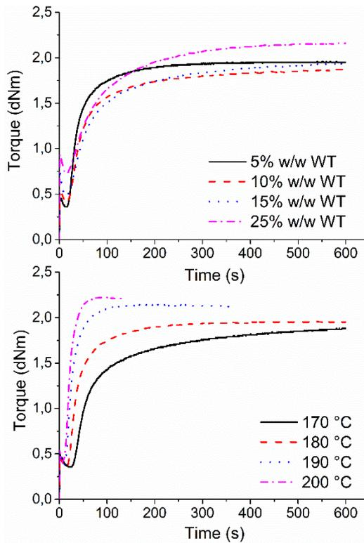
**Figure 5.** Torque graphs of Silicone/Waste Tyre composites
