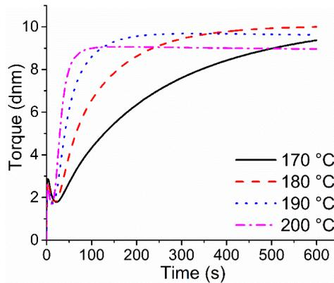
**Figure 1.** MDR test results of EPDM/Waste Tyre Samples
