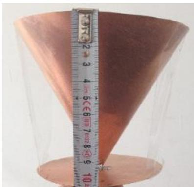
**Figure 9.** Fabricated Antenna.
