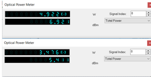
Figure 14. Optical powers of input and output signals measured in Watts and dBm for a fiber length of 10 km, for the hybrid WDM/TDM PON system
