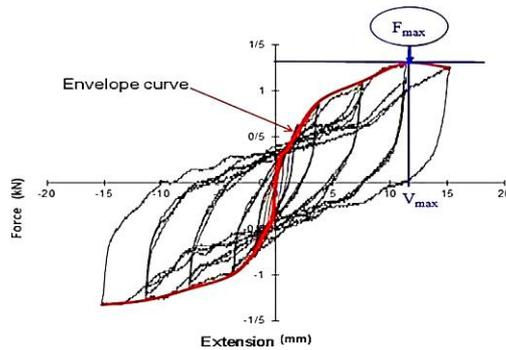
**Figure 5.** Typical cyclical behavior of a bracket connection
