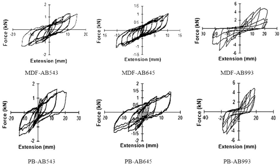
**Figure 8.** Load-displacement hysteresis loop curves of connections under cyclic load
