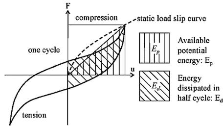
**Figure 6.** Definition of  $E_d$  and  $E_p$  for the determination of the equivalent viscous damping ratio for one cycle
