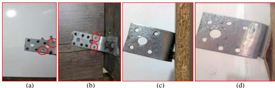
**Figure 9.** Failure modes of connection: screw failure in PB-993 (a) and MDF-993 (B) and panel failure in PB-543 (c) and MDF-645 (d)
