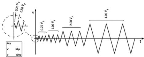
**Figure 3.** Cyclic procedure according to EN 12512
