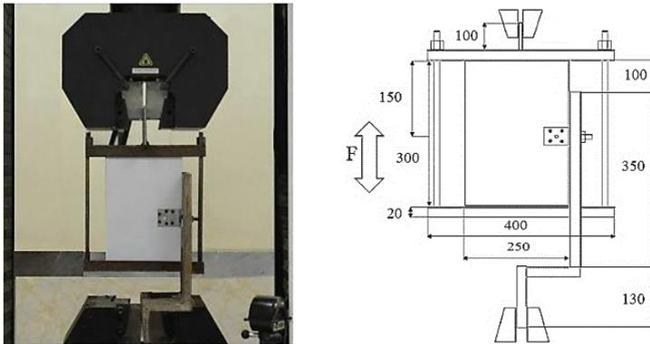
**Figure 2.** Test setup used for monotonic and cyclic loading
