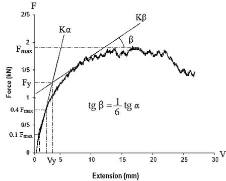
**Figure 4.** Determination of yielding point according to EN 12512
