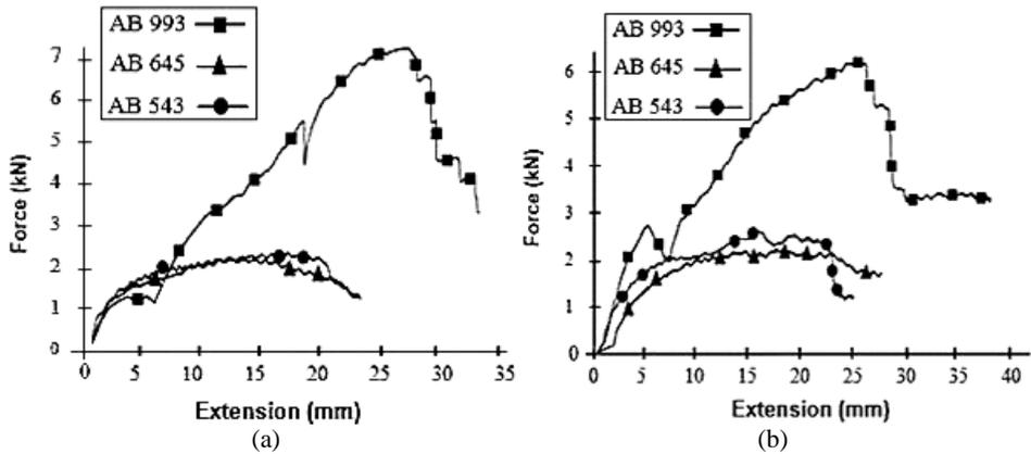
**Figure 7.** Load–displacement curves of connection made of brackets and (a) particleboard and (b) MDF under monotonic loading
