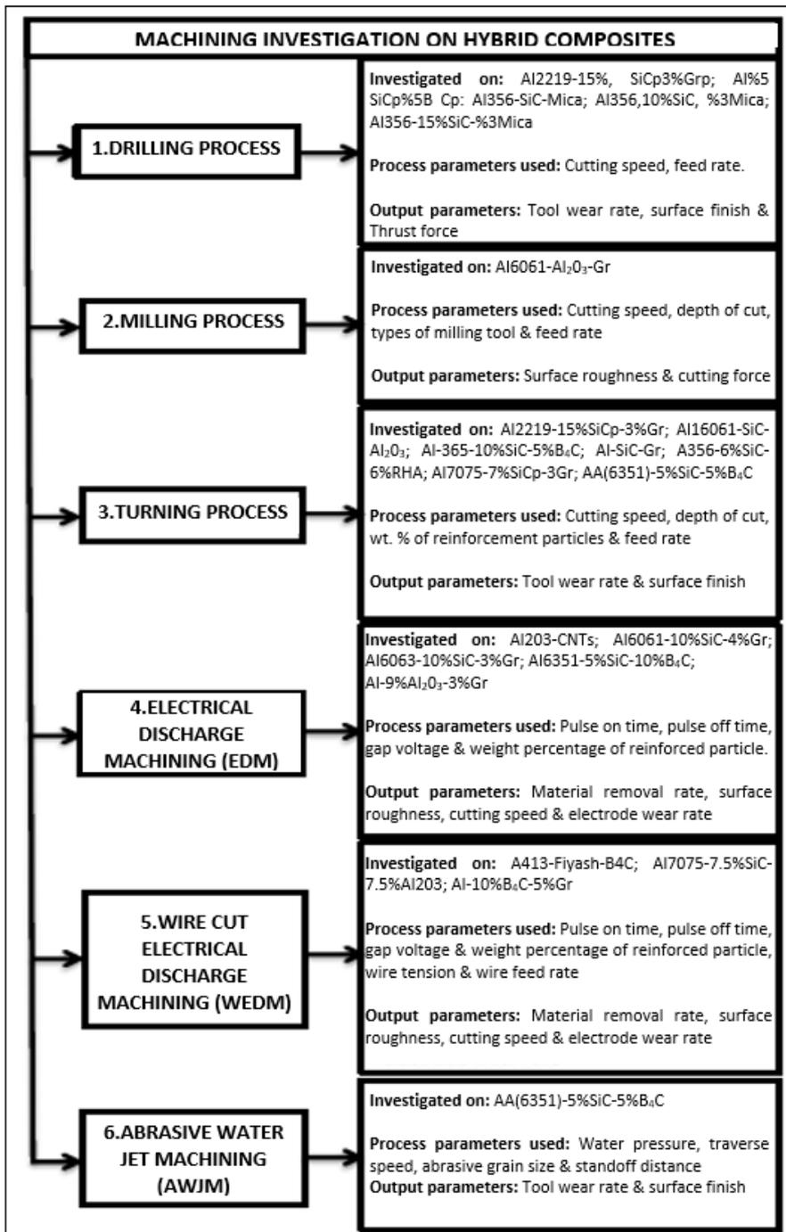
Figure 2.2. Different machining methods and investigations on hybrid composites
