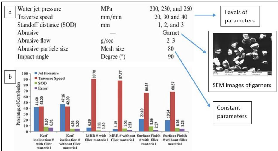
**Figure 3.8.** Cutting parameters (a) and percentage contribution of parameters to the results with regards to kerf structure, MMR and surface finish (b) [87]
