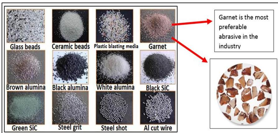
**Figure 2.6.** Abrasive types for AWJC/AWJT applications and close view of garnet grains [47]
