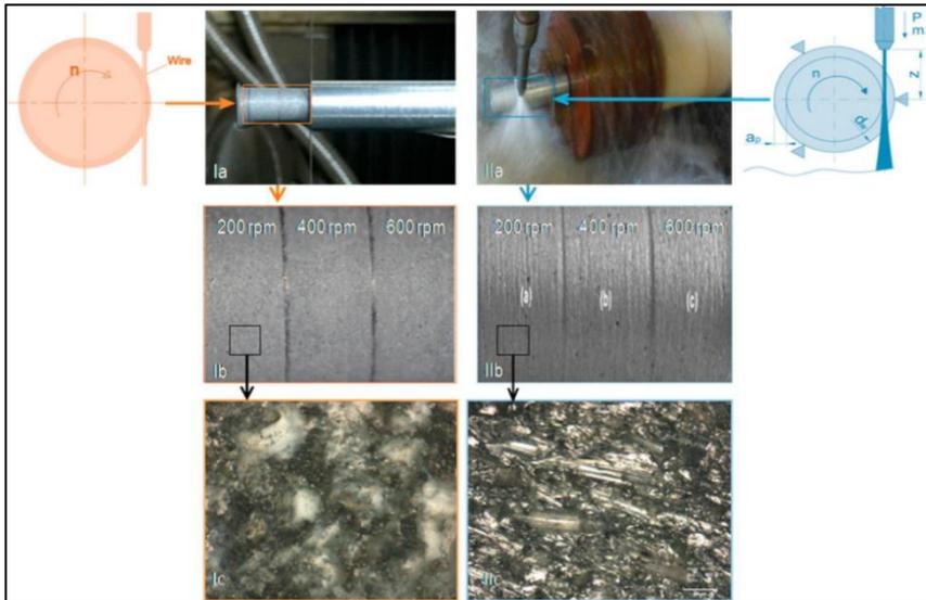
**Figure 3.11.** WED and AWJ turning processes and comparison of machined surfaces in the same rotational speed [90]
