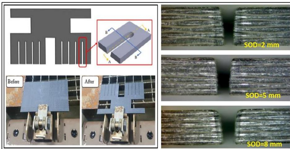
**Figure 3.3.** Cutting design for FRP hybrid specimens and alteration of kerf tapers based on stand-off distance [70]
