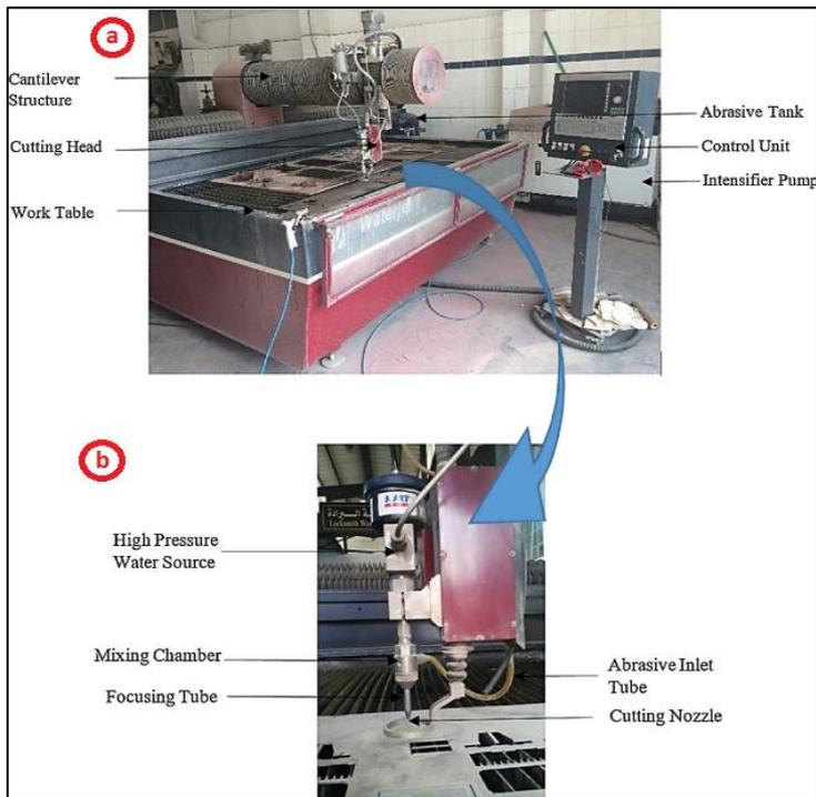
**Figure 2.3.** Real setup of an abrasive waterjet cutting (a) and cutting head (b) [42]
