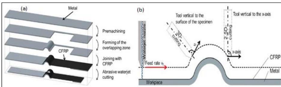
**Figure 3.2.** Specimen preparation steps (a) and different cutting strategies (b) [28]
