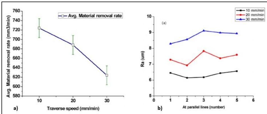
Figure 3.9. Relation between traverse speed and MRR (left) and roughness (right) [88]
