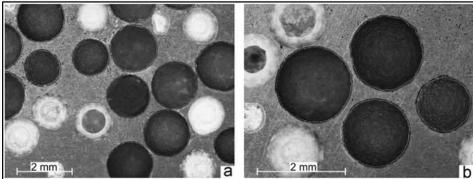
**Figure 3.12.** Microstructure of aluminum/unlike ceramic hollow spheres syntactic foam [15]
