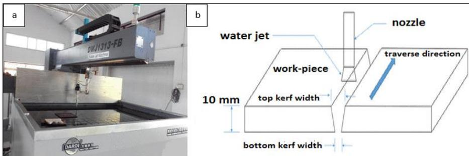
**Figure 3.5.** AWJC setup (a) and kerf geometry (b) [83]
