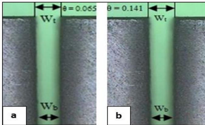
**Figure 3.7.** Kerf taper angles of the different vol. reinforced samples; high (a), low (b) [86]
