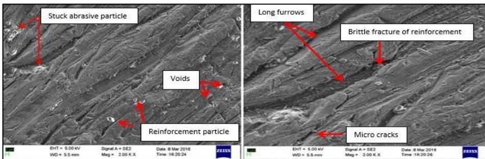
Figure 3.10. SEM images of turned sample surface and some microstructural detections [88]
