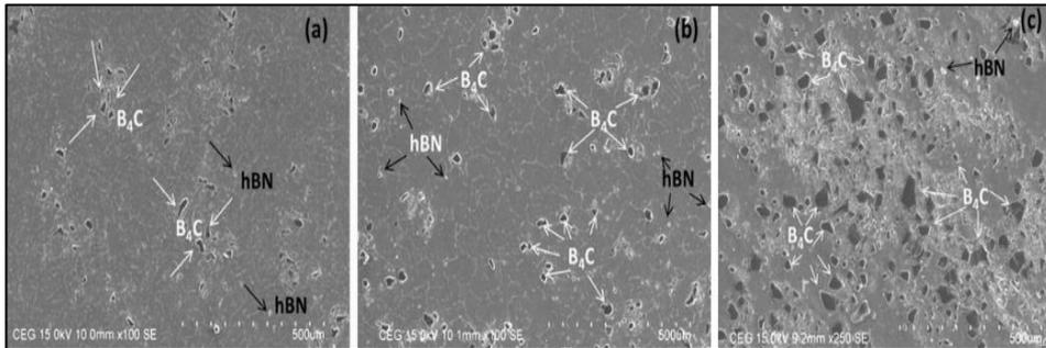
**Figure 3.1.** SEM images of hybrid AMMCs (a) %5 B<sub>4</sub>C, (b) %10 B<sub>4</sub>C, (c) %15 B<sub>4</sub>C [16]
