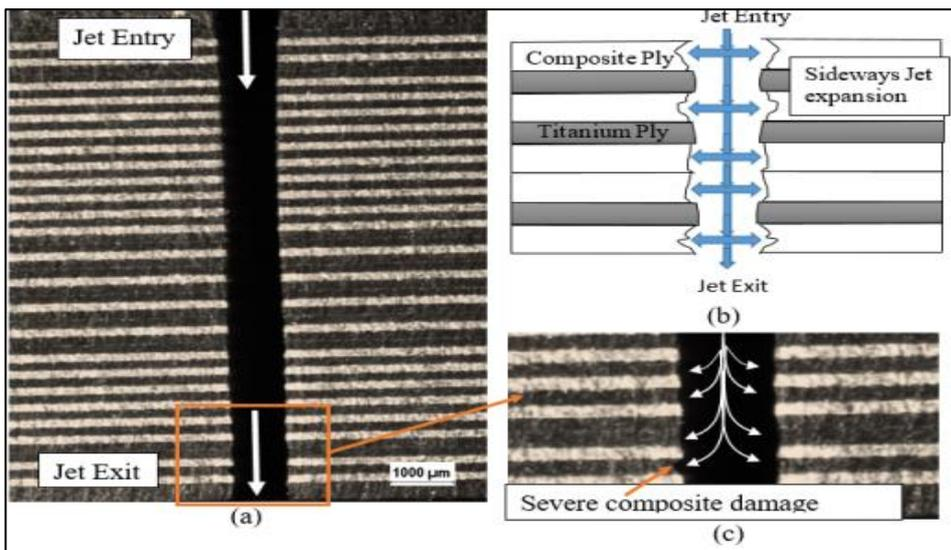
**Figure 3.6.** Kerf characteristics of 10.5 mm thick specimen, (a) jet direction on the kerf wall, (b) schematic view of the kerf, (c) exit kerf [84]
