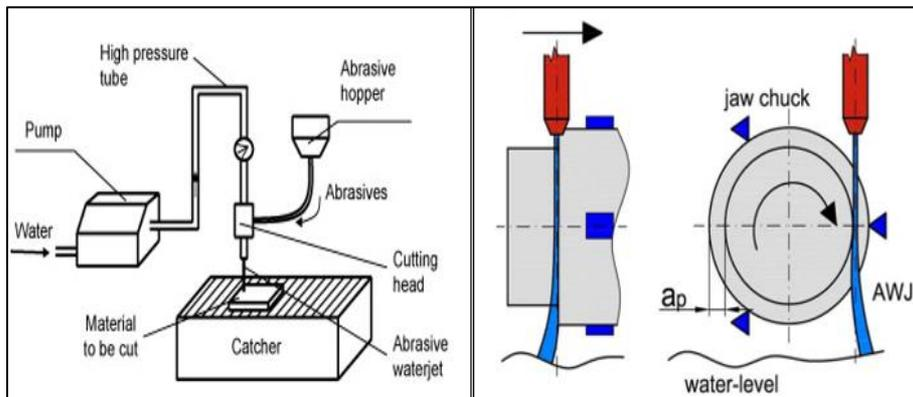
**Figure 2.5.** Schematic view of AWJC (left) and AWJT (right) processes [43], [46]
