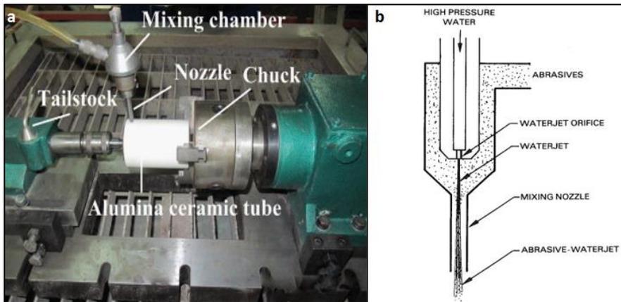
**Figure 2.4.** A real setup example of AWJT system (a) and nozzle system (b) [44]
