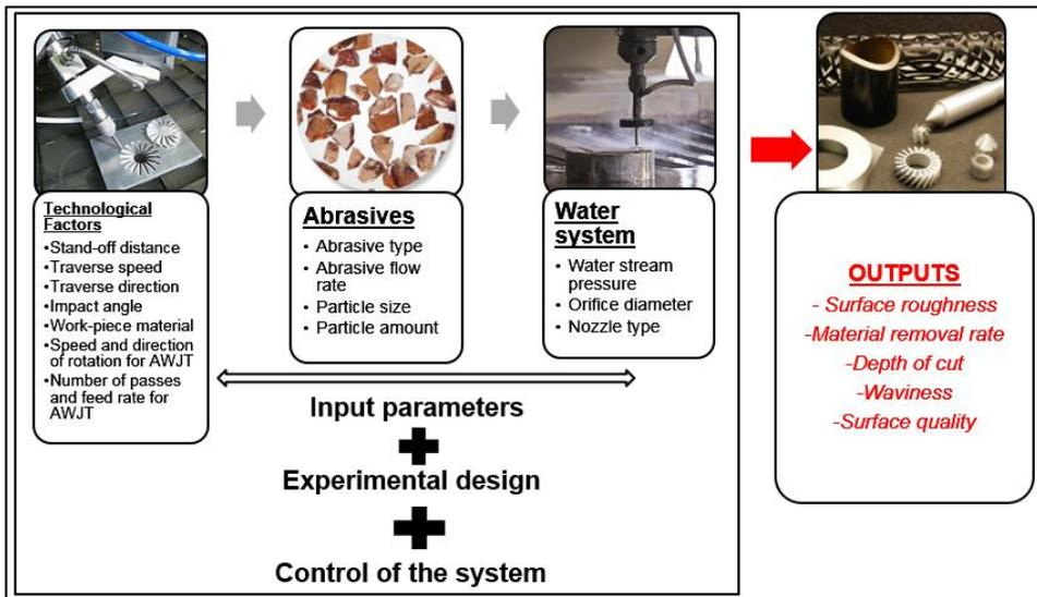
Figure 2.8. Input and output factors for AWJC and AWJT processes [47], [52], [64-69], [72]
