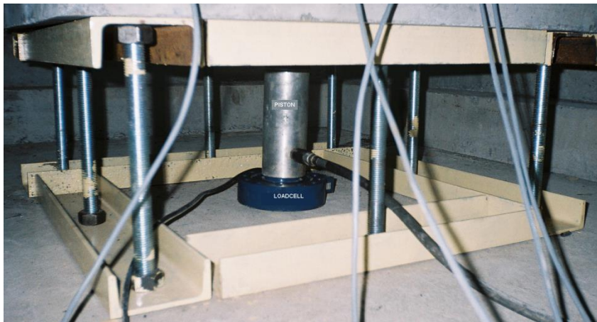
Figure 2. Loading piston and load-cell
