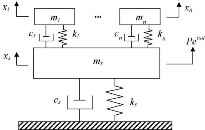
**Figure 1.** Primary structure – MTMD coupled system
