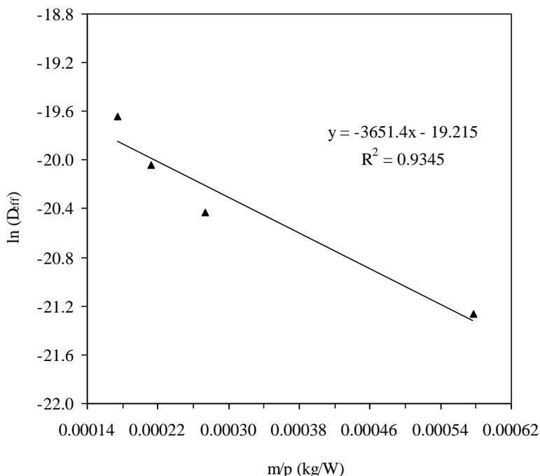
**Figure 5.** Arrhenius-type relationship between effective diffusivity and power levels
