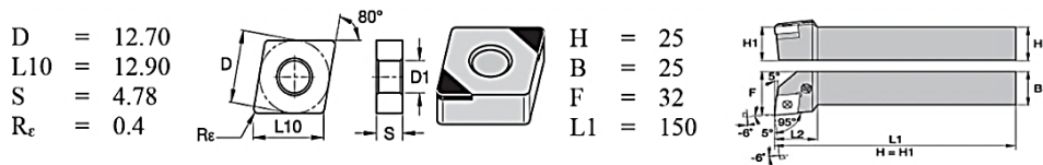
Figure 2. Cutting tools and tool holder used in the turning experiments
