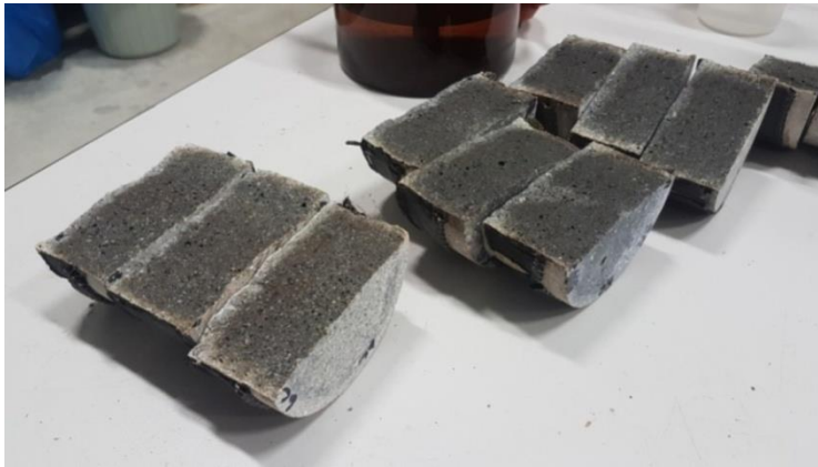
Figure 6. Compositions of samples subjected to chloride impermeability test
