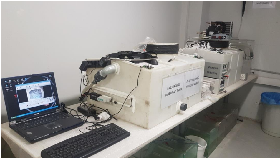
Figure 2. Carbonation experimental setup
