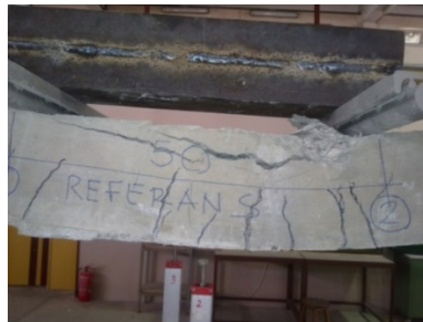
Figure 11. Close view of fracture in CONTROL sample [19]
