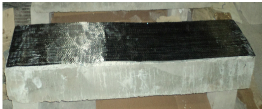
Figure 6. Application of CFRP sheets at flexure section [19]
