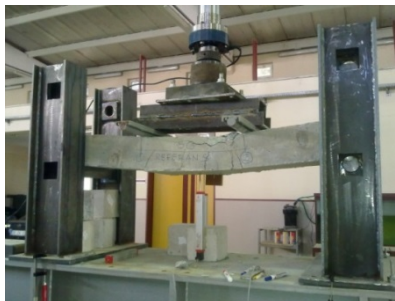
Figure 9. Failure of control sample [19]
