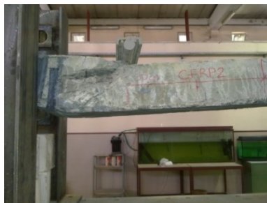
Figure 17. Failure of the three samples strengthened with CFRP sheets [19]
