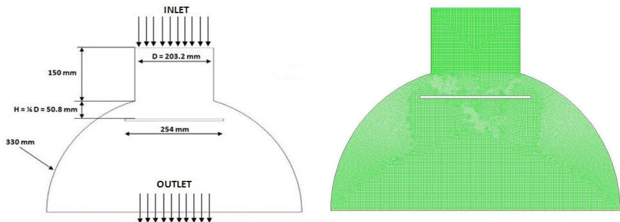
Figure 1. 2-Dimension computational domain and meshed zone
