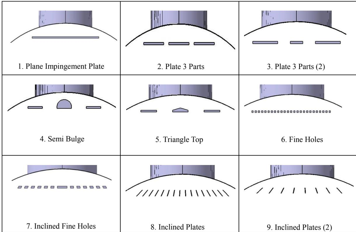
**Figure 6.** 2D Impingement plate geometries
