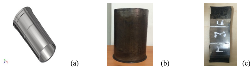
Figure 2. CAD drawing of cylinder liner (a), cylinder liner used in this experimental study (b) and three (3) equal parts (upper-middle-lower) on each section of the cylinder liner used in this experimental study (c).
