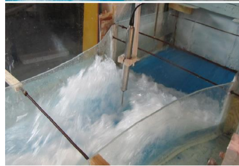
Figure 4. The hydraulic jump in the contractions for Fr_1=7.3
