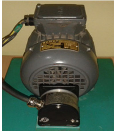
Figure 5. Used three-phase squirrel cage induction motor
