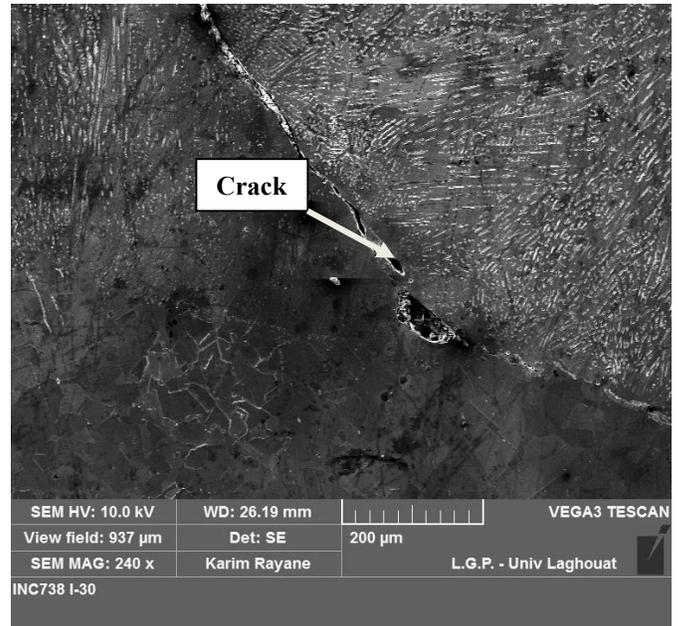
**Figure 5.** SEM observation of the welded joint in fusion zone of welded austenitic stainless steel AISI 304L .
