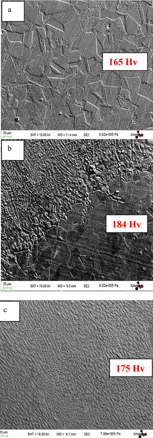
**Figure 2.** SEM observations of the base metal (BM), ( b) the heat affected zone ( HAZ ),and (c) the fusion zone ( FZ) OF austenitic stainless steel AISI 304L after welding.
