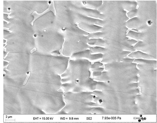
**Figure 3.** High magnification of fusion zone of austenitic stainless steel AISI 304L after welding.
