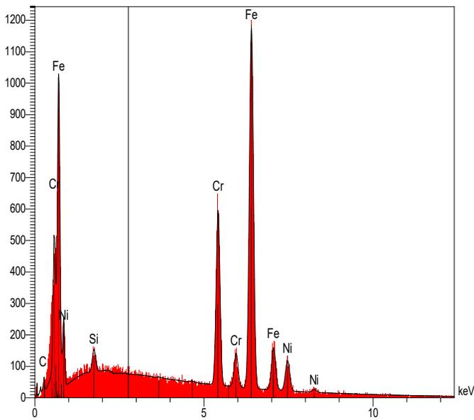
**Figure 1.** EDS spectrum of the base metal austenitic stainless steel AISI 304L.
