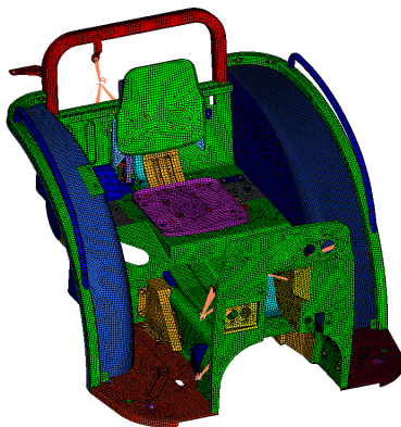
Figure 6. FE Mesh Model for Platform Structure
