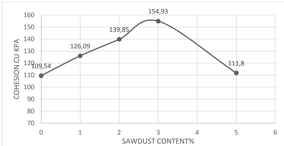
Figure 7. Effect of Sawdust Content on the Cohesion of the soil in the Unconfined Compression test
