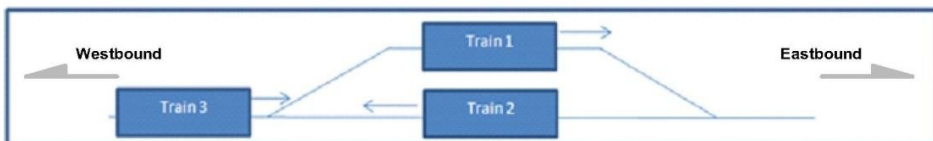
Figure 9. Feasibility will be guaranteed by forcing Train 3 to wait without entering the station until Train 1 leaves the station.
