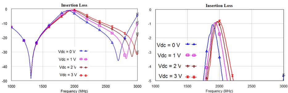
Figure 5e. Insertion loss Response of Filter 1 with Variation of  $V_{DC}$
