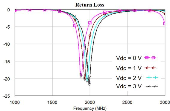
Figure 5a. Varactor capacitance vs. tuning voltage Return Loss Response of Filter 1 by variation of DC Voltage.
