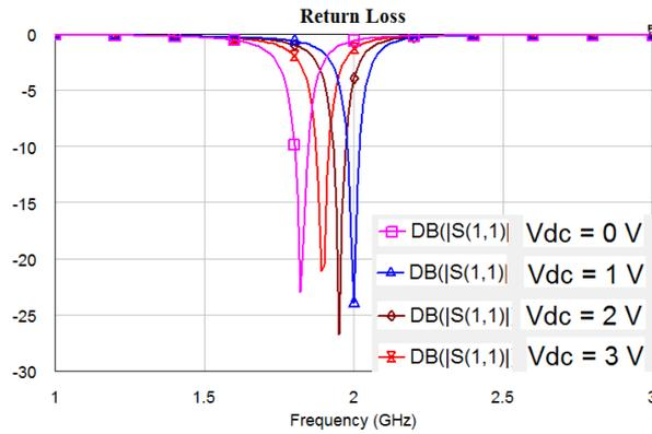
**Figure 5b.** Return Loss Response of Filter 2 by variation of DC Voltage.
