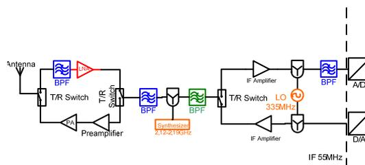
**Figure 1.** An example schematic for Radio System Architecture
