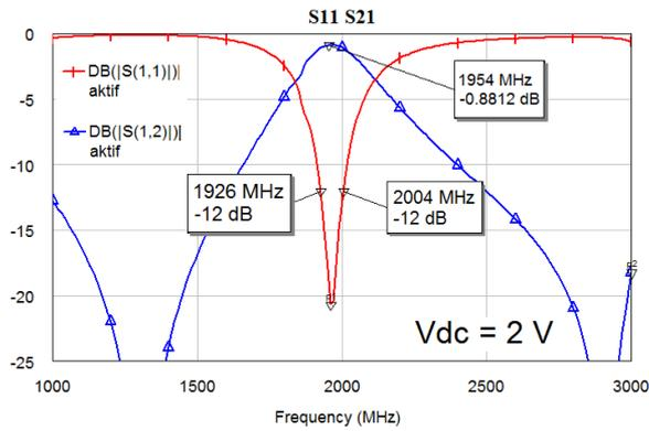
**Figure 5c.** Bandwidth of filter 1, V<sub>DC</sub>=2V with reference of -12dB
