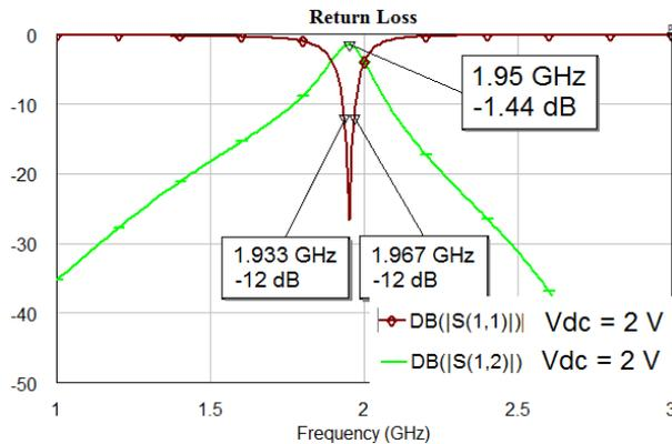
**Figure 5d.** Bandwidth of filter 2, V<sub>DC</sub>=2V with reference of -12dB
