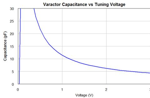
Figure 4. Varactor capacitance vs. tuning voltage
