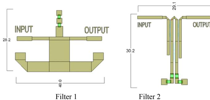
**Figure 2.** Simple tunable filter structure
