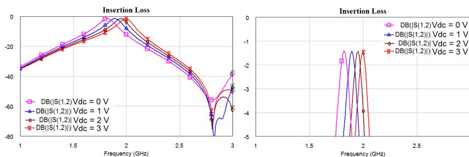
Figure 5f. Insertion loss Response of Filter 2 with Variation of  $V_{DC}$
