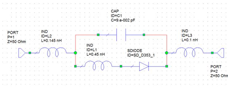
**Figure 3.** Lumped model of the varactor (BBY58-02)
