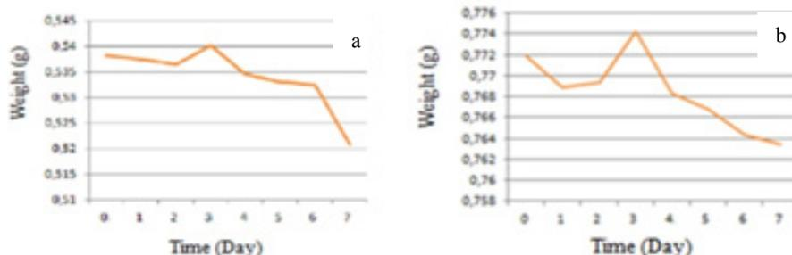
**Figure 4.** Weight loss of bioactive glass samples in TRIS solution a) 45S5-SrR b) 45S5-SrC
