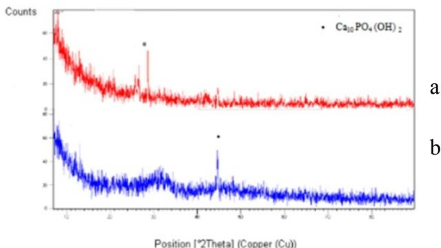
Figure 2. XRD patterns of 45S5-SrR a) before SBF b) on 28th day in SBF
