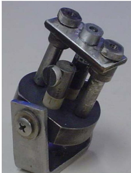
Figure 1. Photo of the cathode showing the filament placed inside the Wehnelt
