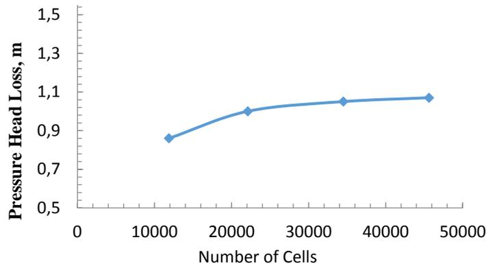
Figure 2(a). Grid independence test
