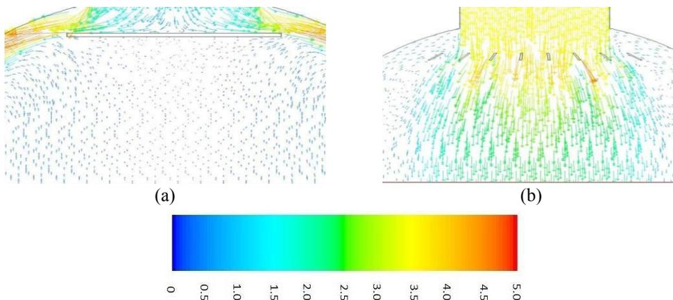
**Figure 7.** Velocity Vectors for (a) Unmodified and (b) Modified Designs
