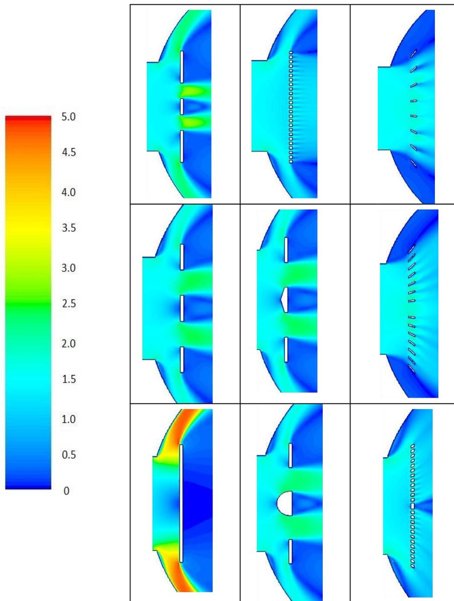
**Figure 8.** Velocity contours for modified plate designs
