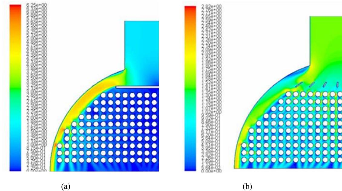
Figure 11. Velocity contours with (a) Unmodified (b) Modified Plate geometries
