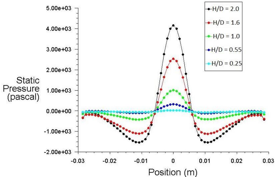
Figure 3. Effect of H/D ratio on the pressure distribution
