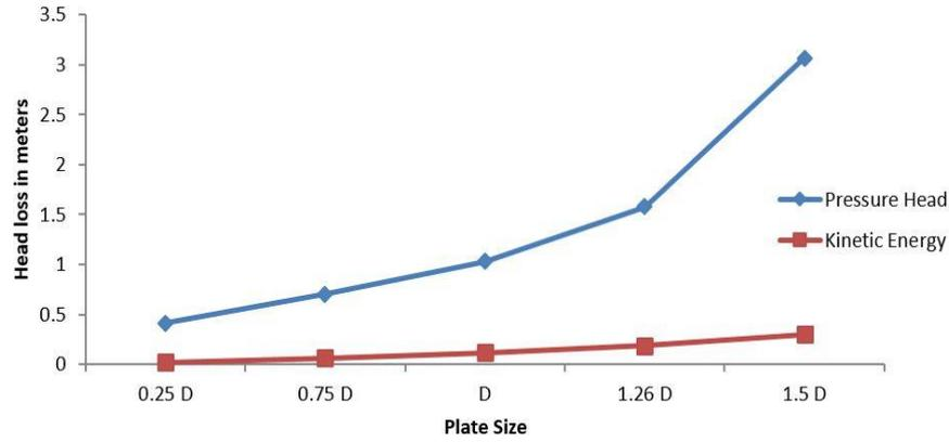
**Figure 4.** Variation of pressure head and kinetic energy loss with plate size
