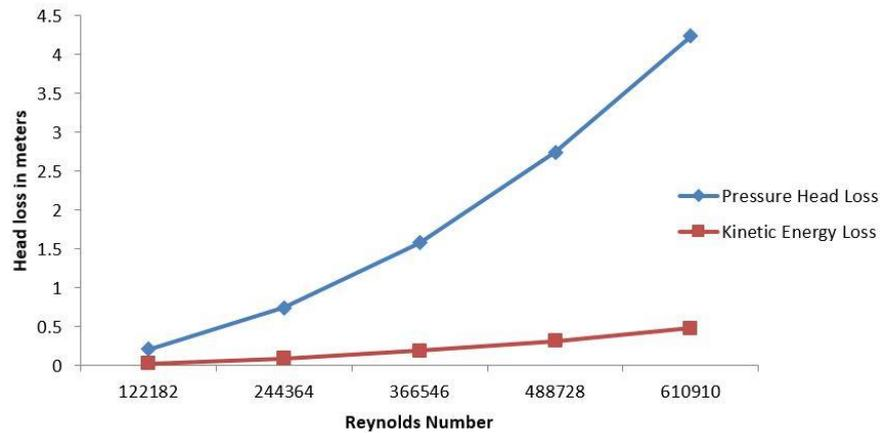
**Figure 5.** Variation of pressure head loss and kinetic energy head loss with Reynolds number
