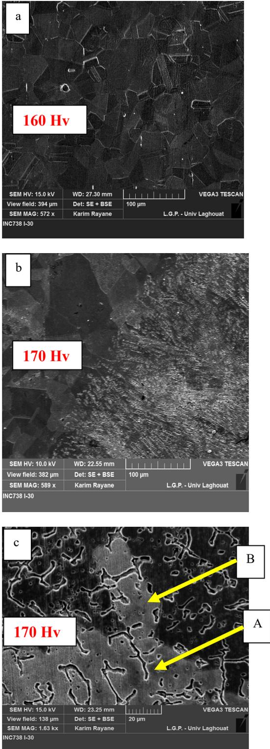
**Figure 6.** SEM observations of the base metal (BM), ( b ) the heat affected zone ( HAZ ) , and (c) the fusion zone ( FZ) after annealing at 300°C for 60 min.
