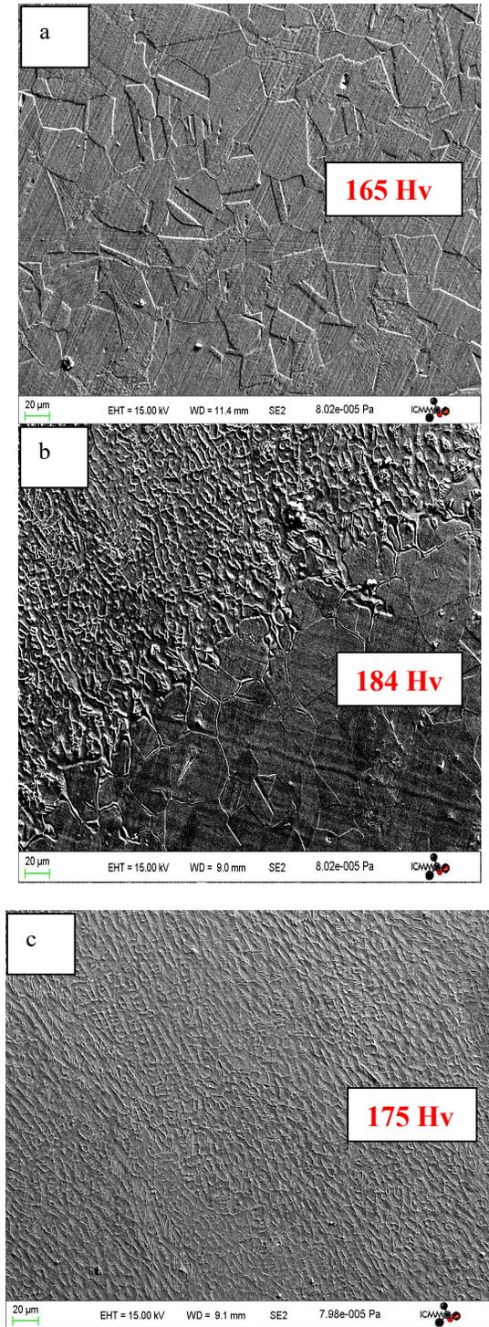
**Figure 2.** SEM observations of the base metal (BM), ( b) the heat affected zone ( HAZ ),and (c) the fusion zone ( FZ) OF austenitic stainless steel AISI 304L after welding.
