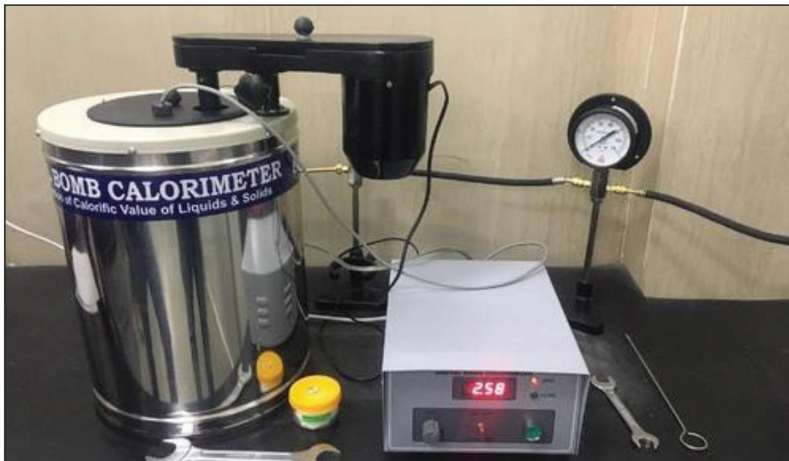
Figure 5. Bomb calorimeter apparatus for calorific value measurement of MSW.
