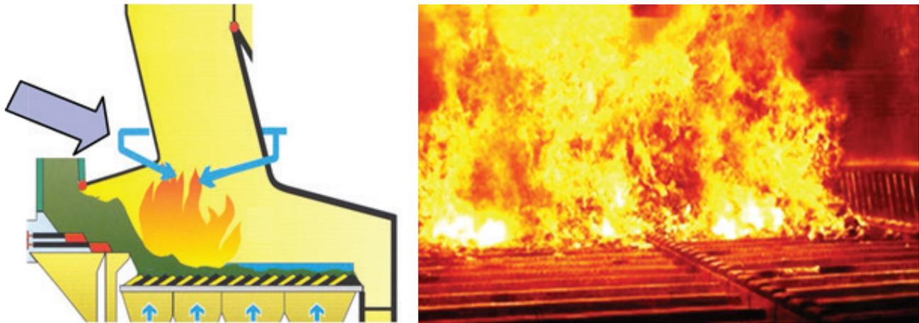
**Figure 7.** Inside view of the solid waste combustion chamber by the infrared camera.
