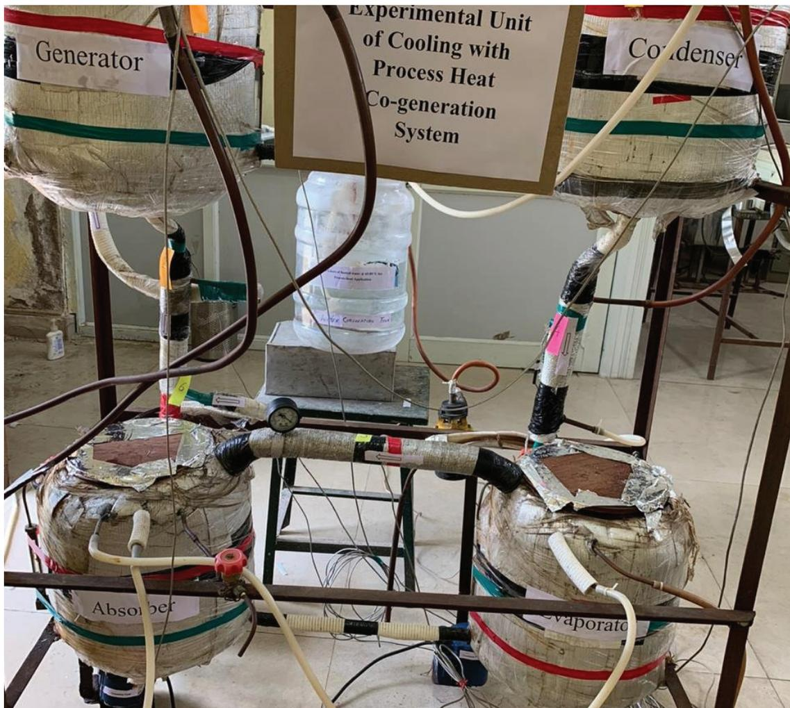
**Figure 3.** Practical test facility of the vapor absorption system.
