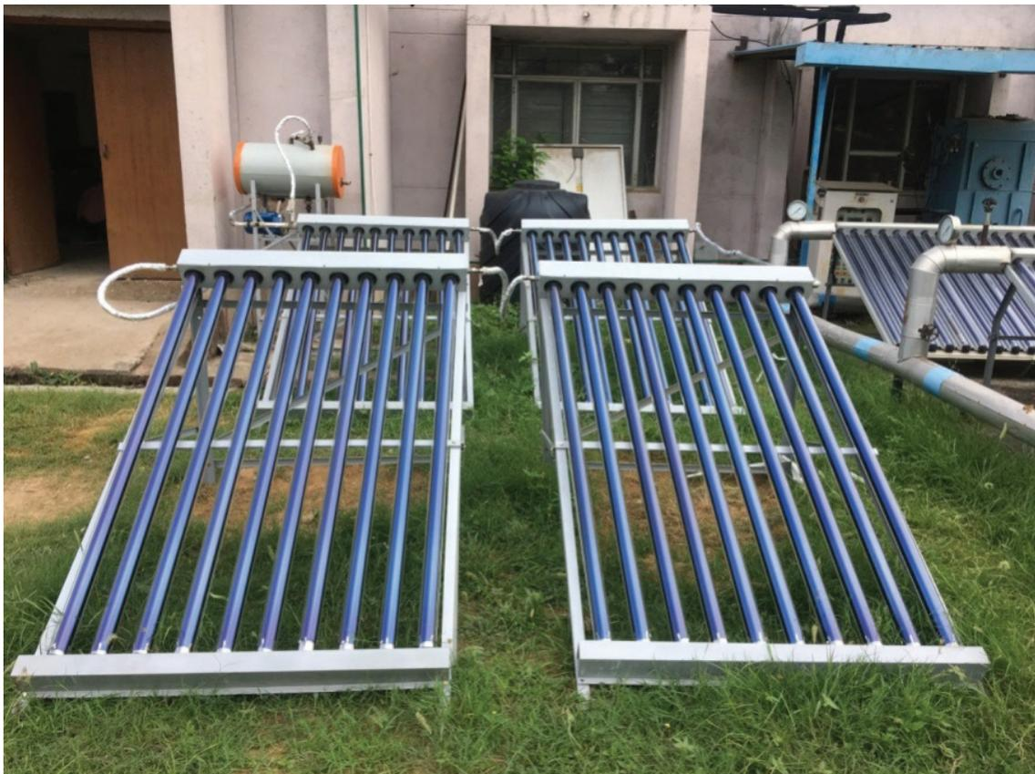
**Figure 4.** A photographic view of the Evacuated Tube Collector used in the experiments.
