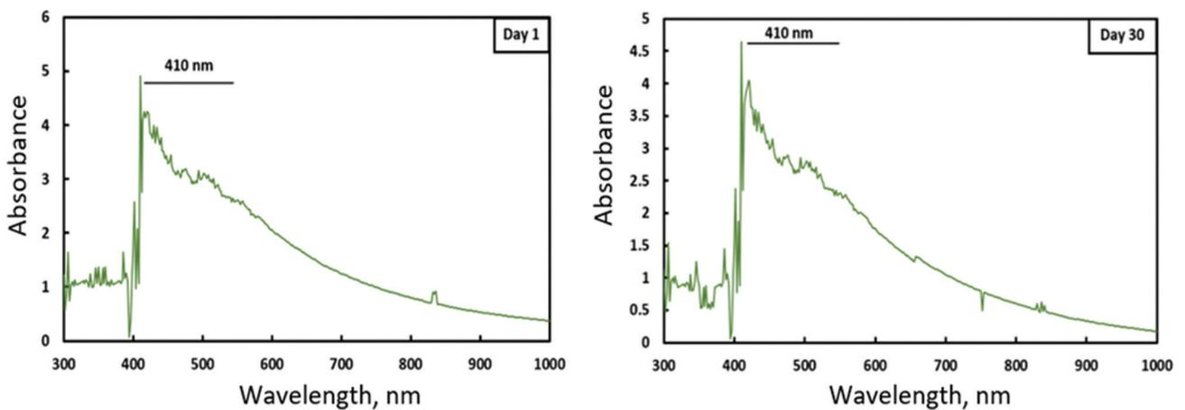
Figure 11. TiO<sub>2</sub>-POE nanolubricant absorbance value comparison (a) day 1 and (b) day 30 from sample 6 with 120 min ultrasonication treatment.
