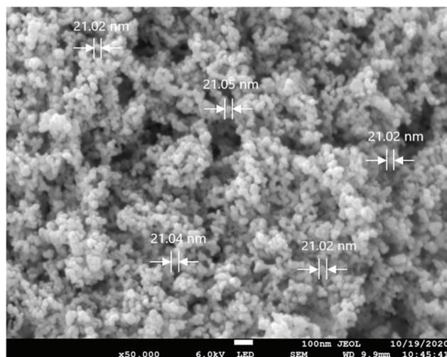
**Figure 4.**  $\text{TiO}_2$  Nanoparticles morphology in 50,000 magnifications.
