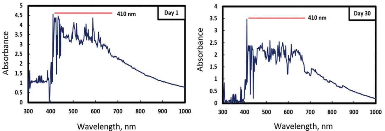
**Figure 9.** TiO<sub>2</sub>-POE nanolubricant absorbance value comparison (a) day 1 and (b) day 30 from sample 3 with 60 min ultrasonication treatment.
