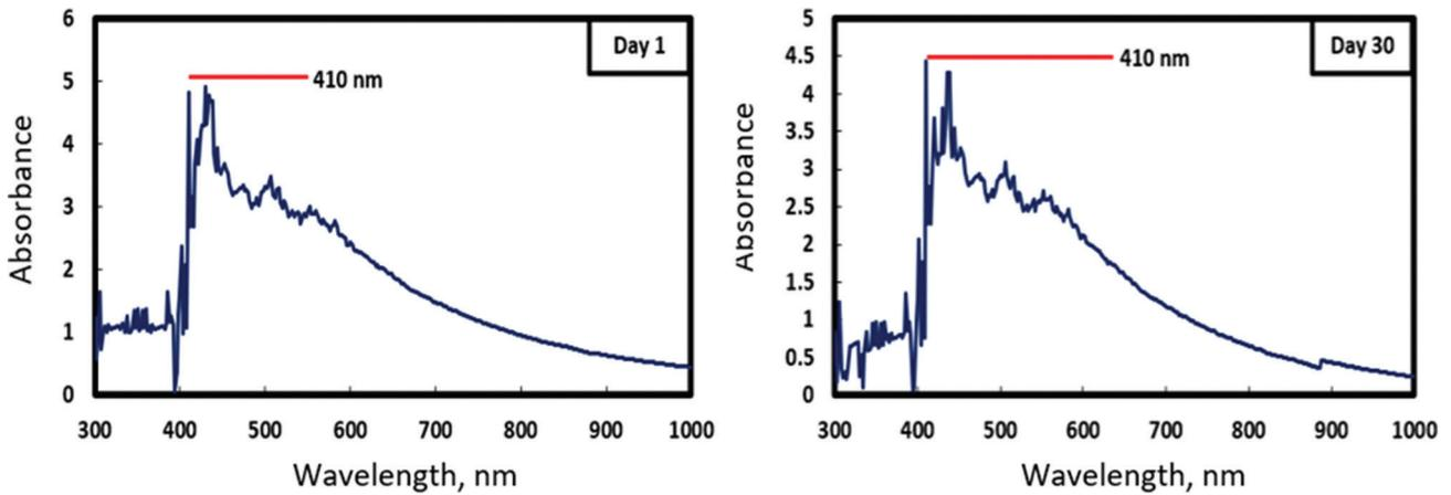
Figure 10. TiO<sub>2</sub>-POE nanolubricant absorbance value comparison (a) day 1 and (b) day 30 from sample 5 with 100 min ultrasonication treatment.
