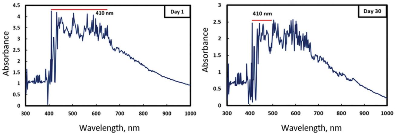
**Figure 8.** TiO<sub>2</sub>-POE nanolubricant absorbance value comparison (a) day 1 and (b) day 30 from sample 2 with 40 min ultrasonication treatment.
