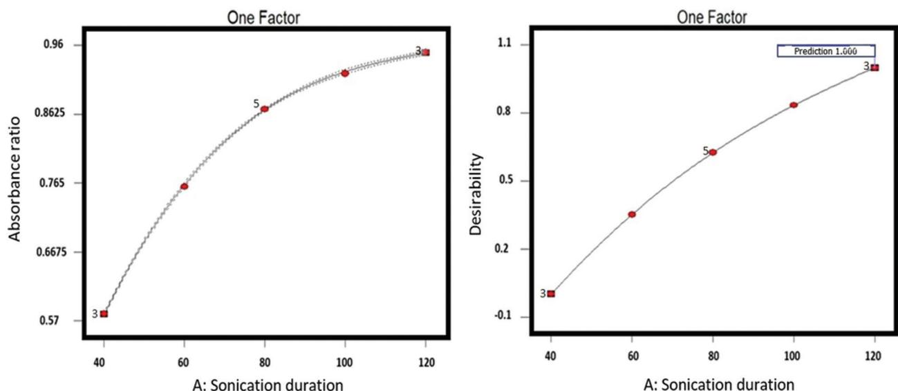
Figure 16. Plot of (a) absorbance ratio as the dependent of sonication and (b) desirability in a one factor at a time in day 30<sup>th</sup>.
