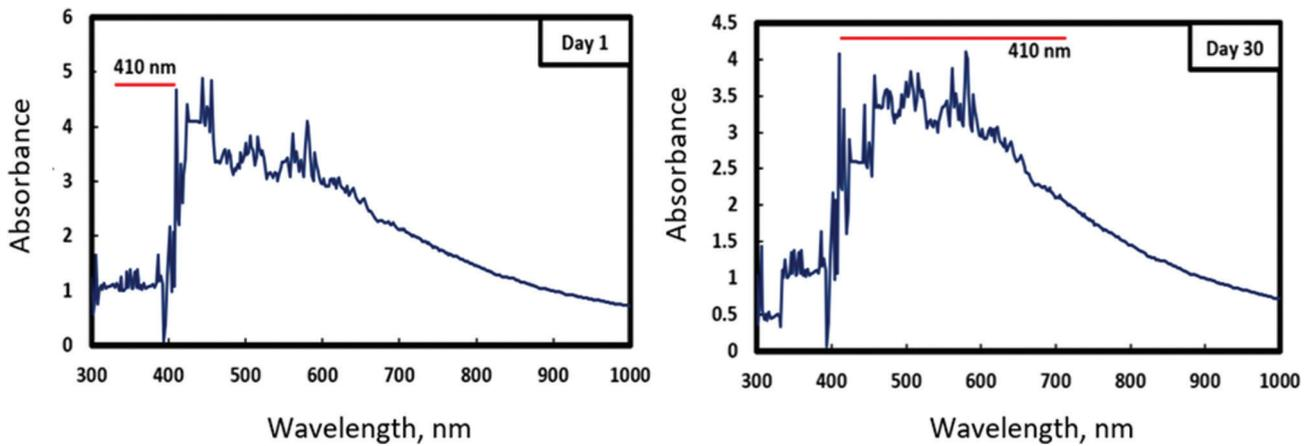
Figure 10. TiO<sub>2</sub>-POE nanolubricant absorbance value comparison (a) day 1 and (b) day 30 from sample 4 with 80 min ultrasonication treatment.
