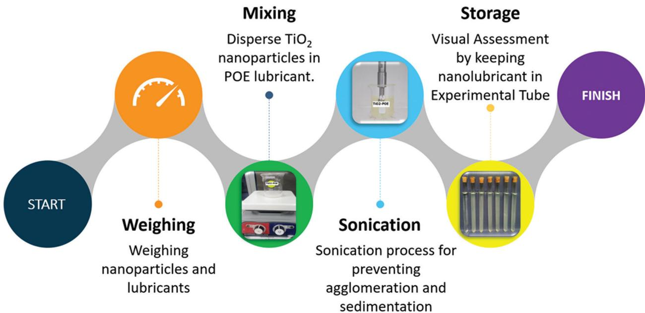
**Figure 1.** Schematic diagram of TiO<sub>2</sub>-POE nanolubricants preparation using a two-step method.
