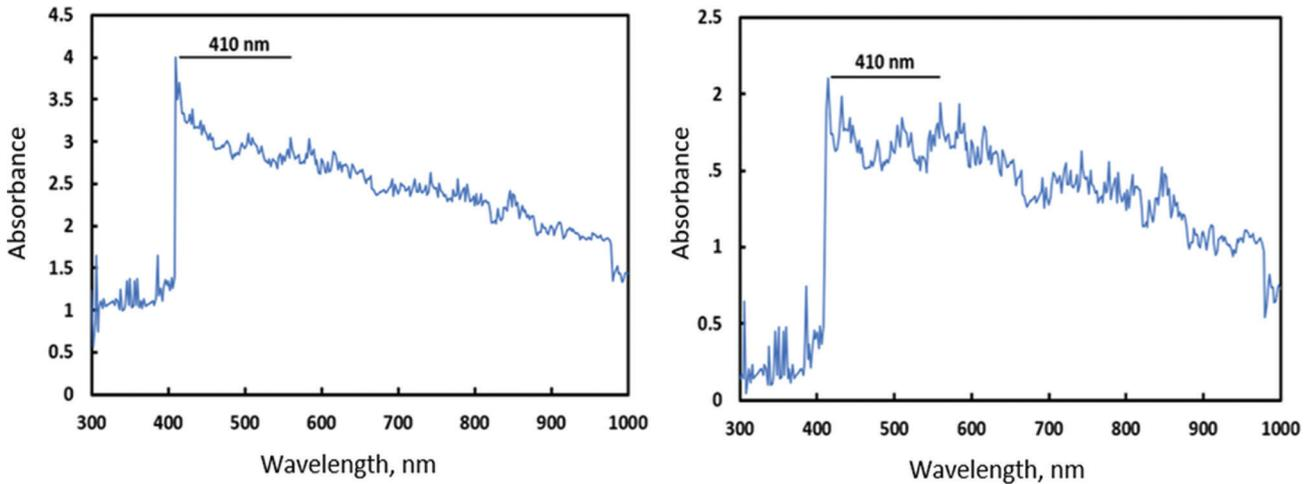
Figure 7. TiO<sub>2</sub>-POE nanolubricant absorbance value comparison (a) day 1 and (b) day 30 from sample 1 with 0 min ultrasonication treatment.
