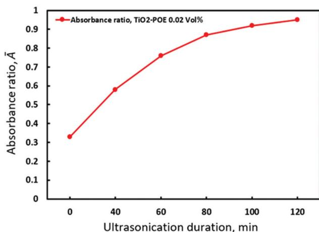
**Figure 12.** TiO<sub>2</sub>-POE nanolubricant absorbance ratio as a dependent of ultrasonication duration.
