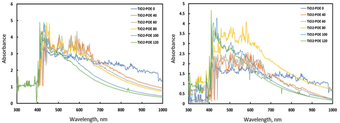
Figure 6. TiO<sub>2</sub>-POE nanolubricant absorbance value comparison (a) day 1 and (b) day 30 from all samples.
