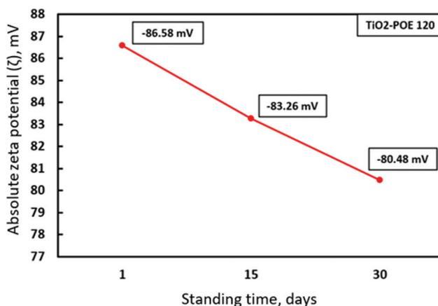
**Figure 13.** TiO<sub>2</sub>-POE nanolubricant absolute zeta potential from sample 6.
