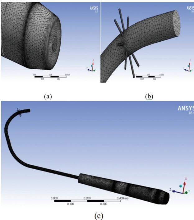
**Figure 6.** Meshing of silencer (a) Closer View at end of silencer. (b) Closer view at air injection. (c) Overall silencer mesh for single air injection plane.
