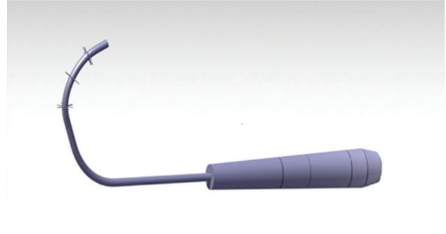
**Figure 5.** Modified silencer model with air injection in three planes.
