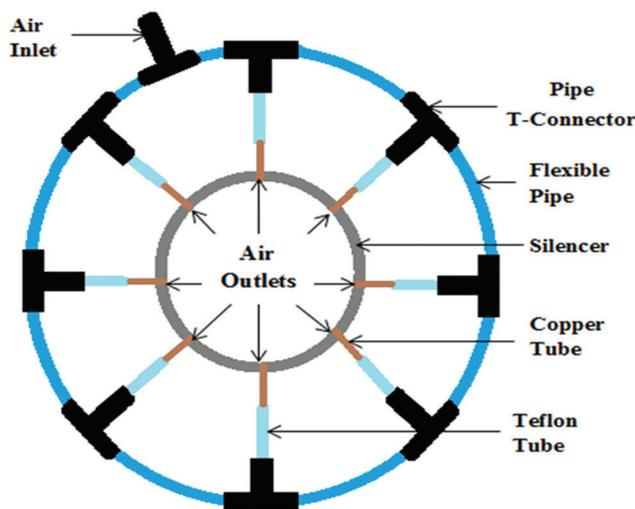
Figure 3. Radial air injection arrangement.
