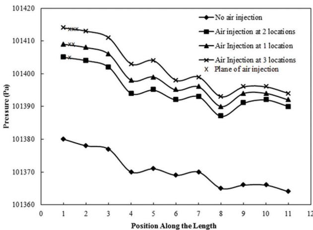
**Figure 11.** Hydrodynamic pressure distribution along the length of silencer.
