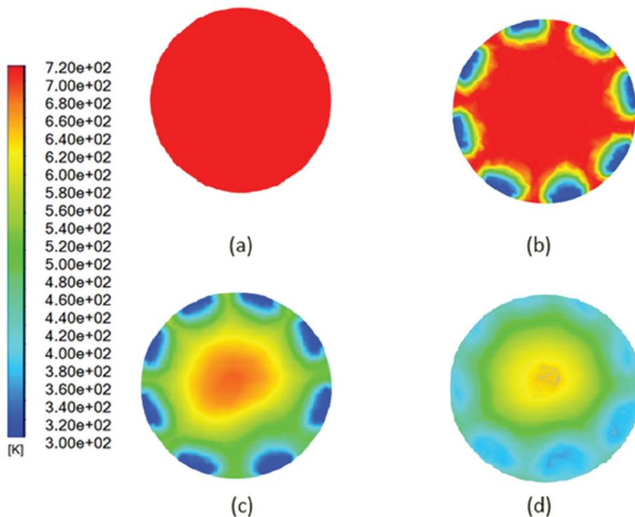
Figure 14. Temperature contour of silencer cross section for air injection at two planes.
