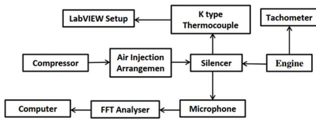
Figure 2. Line Diagram of experimental setup.
