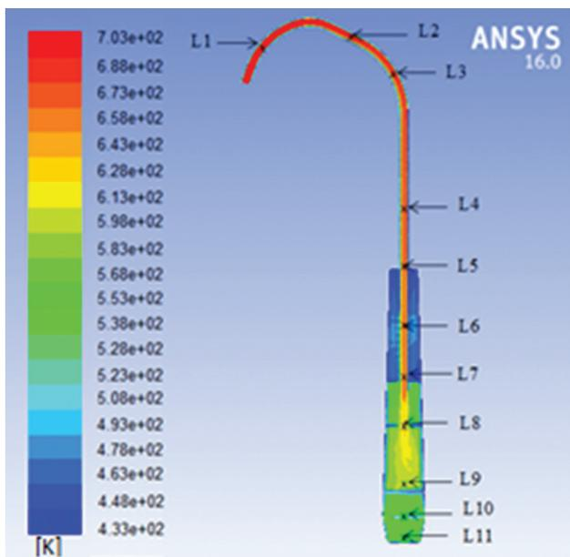
**Figure 10.** Temperature variation plot of Standard Silencer with reference points.
