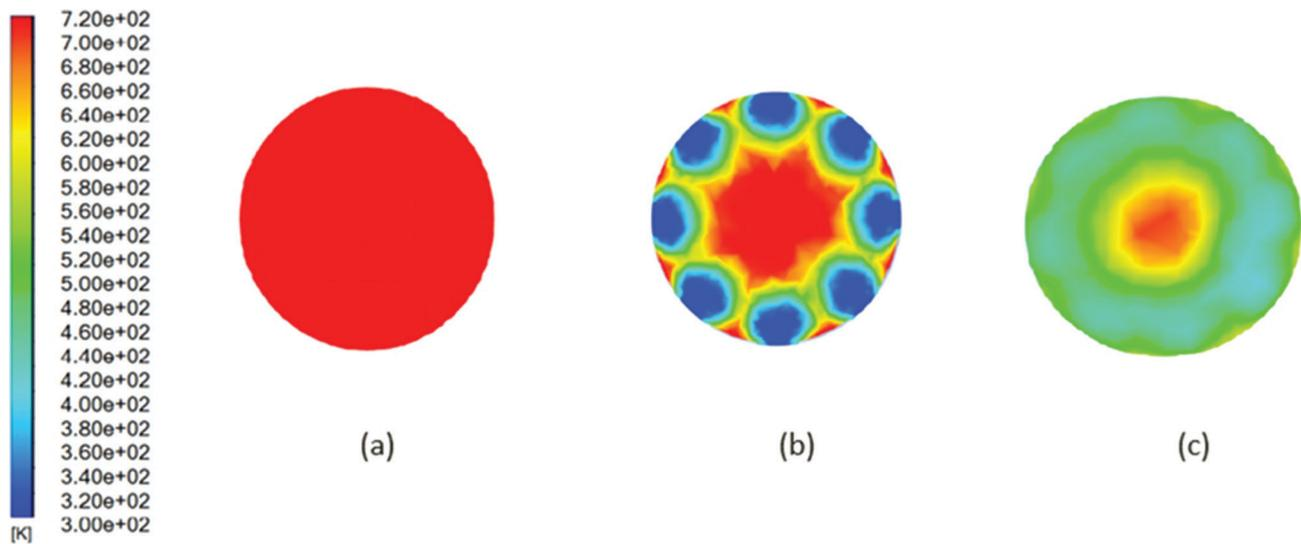
Figure 13. Temperature contours of silencer cross section for air injection at one plane.
