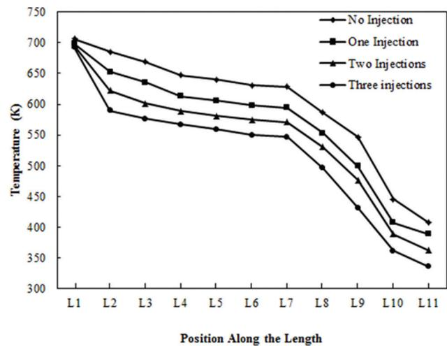
**Figure 12.** Temperature distributions along the length of silencer.
