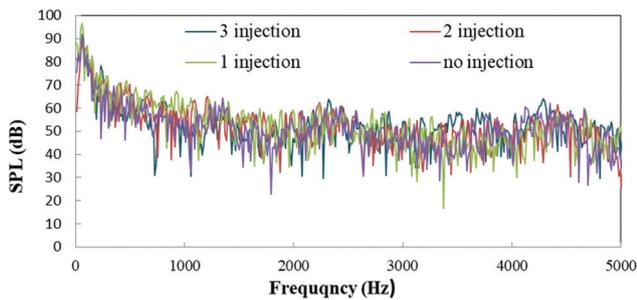
**Figure 7.** Frequency spectra for engine running at 3000 rpm with air injection at one, two and three planes.
