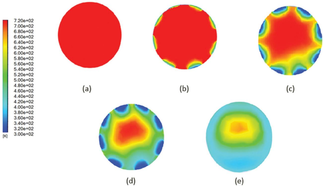
Figure 15. Temperature contours of silencer cross section for air injection at three planes.
