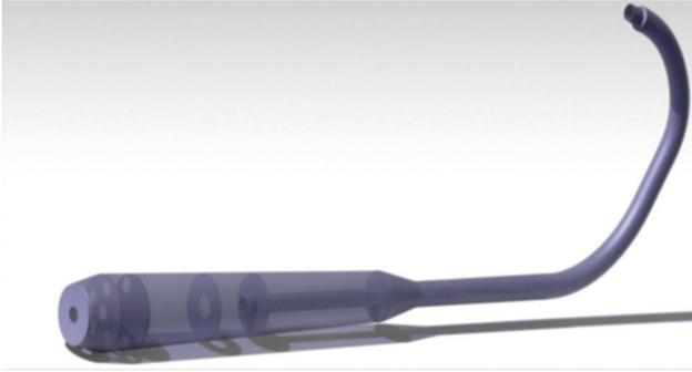
**Figure 4.** 3D model of standard silencer.
