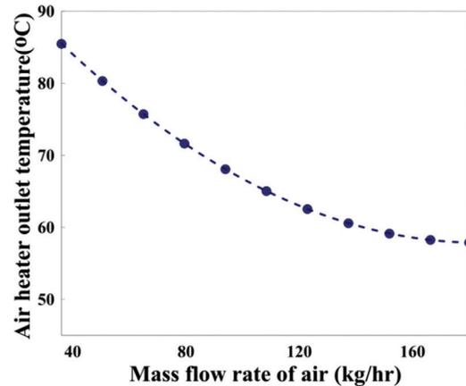
Figure 6. Effect of air mass flow rate on outlet temperature of air.
