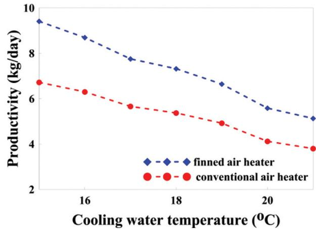
Figure 9. Cooling water temperature vs productivity.
