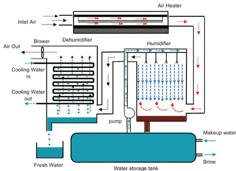
Figure 2. Proposed humidification – dehumidification desalination system.
