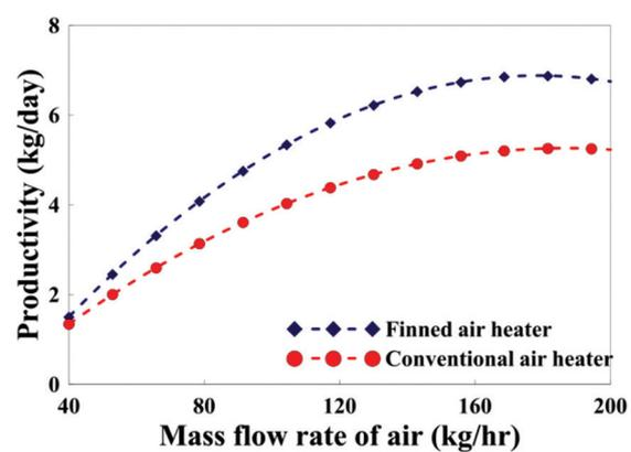
Figure 7. Mass flow rate of air vs Productivity.
