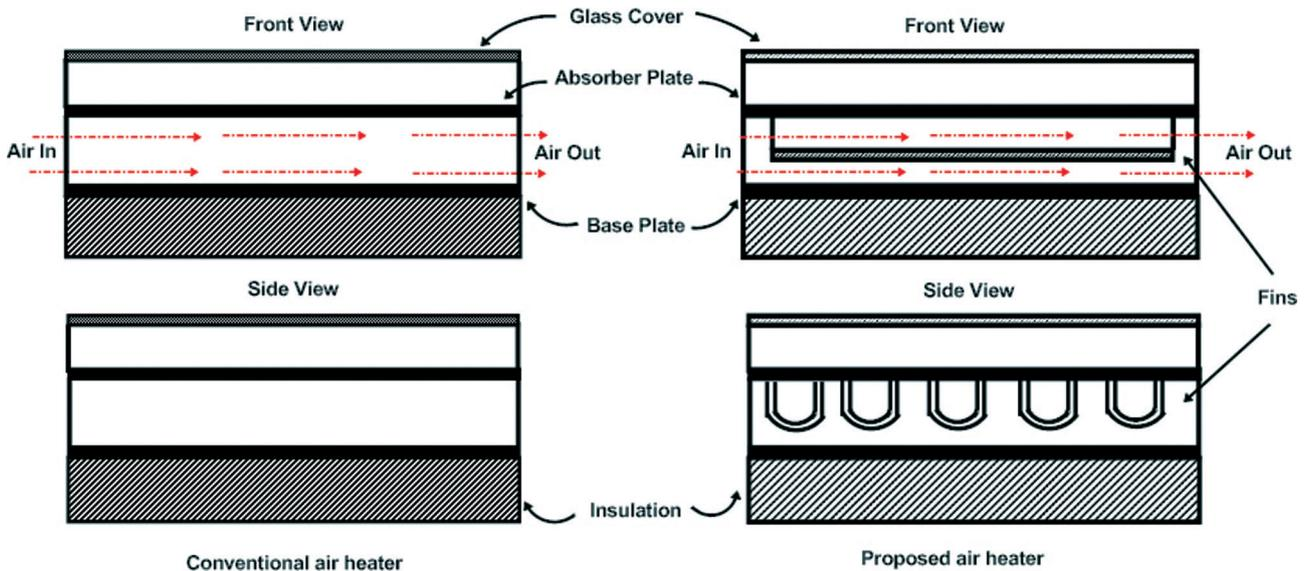
**Figure 1.** Conventional and proposed solar air heater with U - shaped longitudinal fins.
