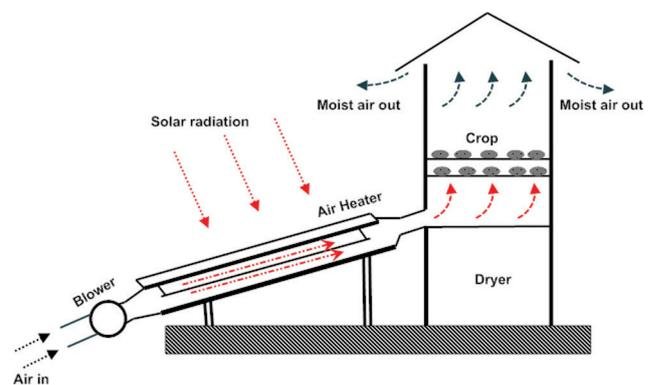
**Figure 3.** Proposed indirect solar drying system.
