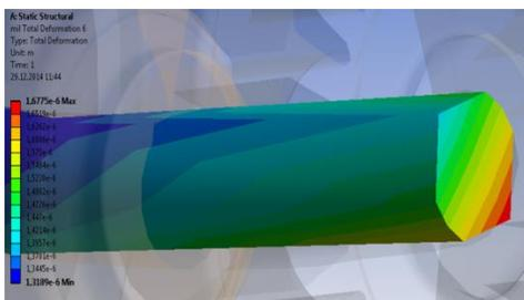
**Figure 20.** The total deformation of the shaft part when the shaft radius of the landing gear is 36 mm and second model.
