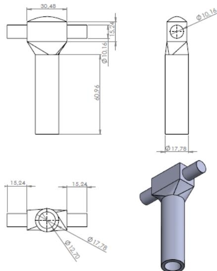
Figure 2. Cylinder of landing gear
