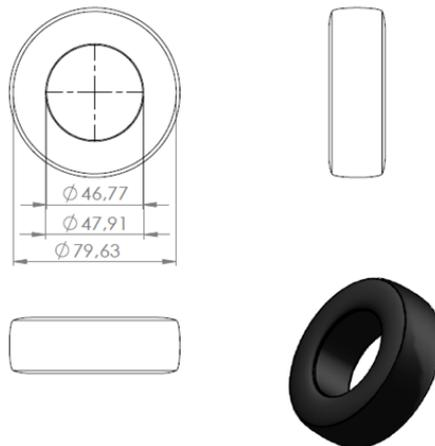
**Figure 5.** The wheel of the landing gear
