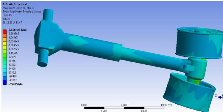
**Figure 13.** First model and maximum stresses in 36 mm landing gear
