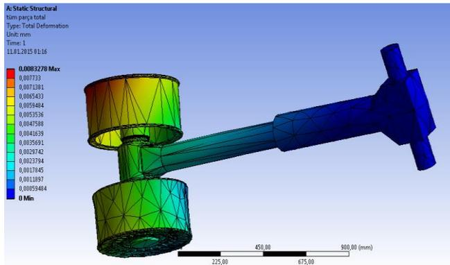
Figure 15. Second model and total deformation of 52 mm landing gear
