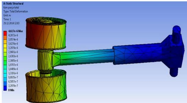
**Figure 12.** First model and total deformation in the 52 mm landing gear
