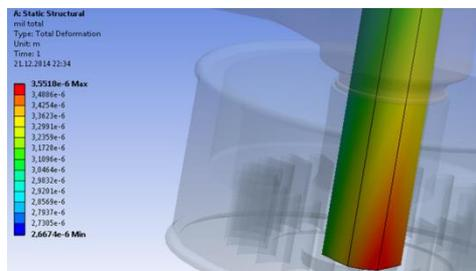
**Figure 21.** The total deformation of the shaft part when the shaft radius of the landing gear is 52 mm and first model.
