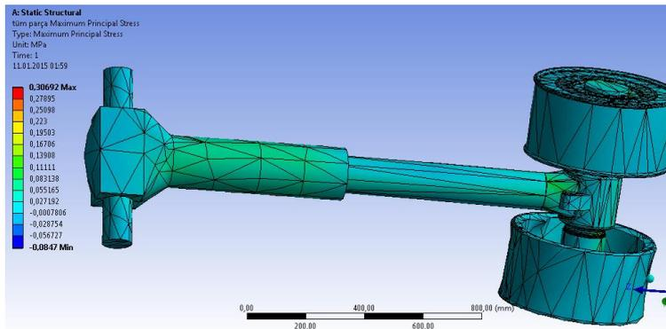
Figure 16. Second model and maximum stresses of 52 mm landing gear
