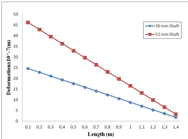
Figure 23. 1st Model-Length-Deformation amount
