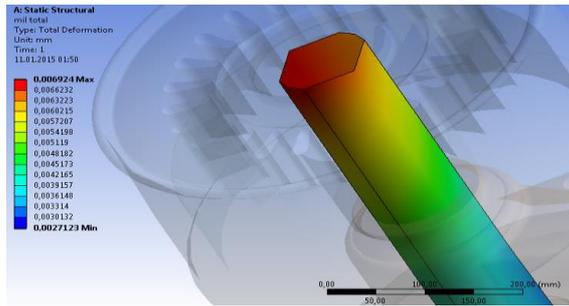
Figure 22. The total deformation of the shaft part when the shaft radius of the landing gear is 52 mm and second model.
