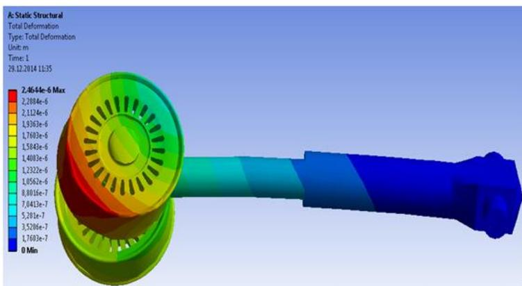
**Figure 11.** First model and total deformation in the 36 mm landing gear
