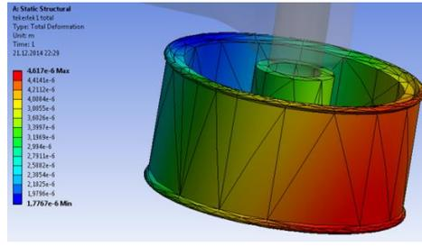
**Figure 18.** The total deformation of the rim part when the shaft radius of the landing gear is 52 mm and first model.
