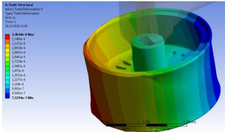
**Figure 17.** The total deformation of the rim part when the shaft radius of the landing gear is 36 mm and first model.
