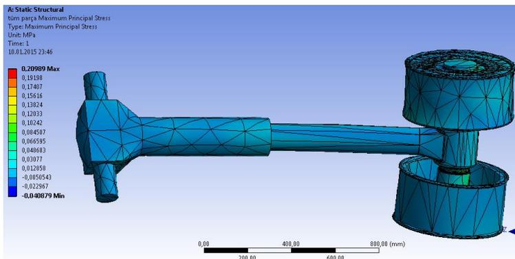
**Figure 14.** First model and maximum stresses in 52 mm landing gear
