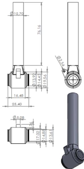
Figure 1. The piston of the landing gear
