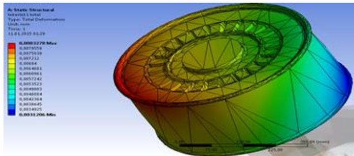
**Figure 19.** The total deformation of the rim part when the shaft radius of the landing gear is 52 mm and second model.
