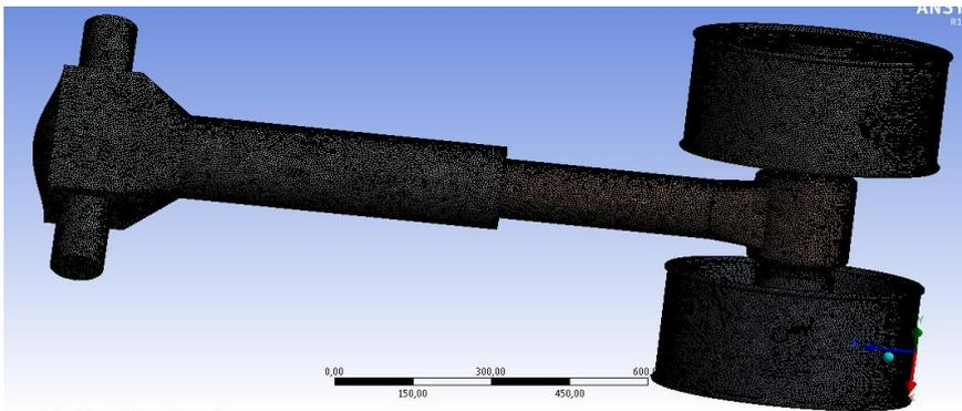
**Figure 8.** Mesh structure of the landing gear
