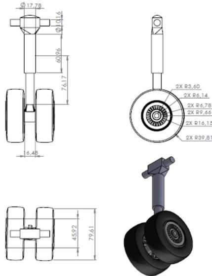
**Figure 6.** Technical picture of the auxiliary landing gear
