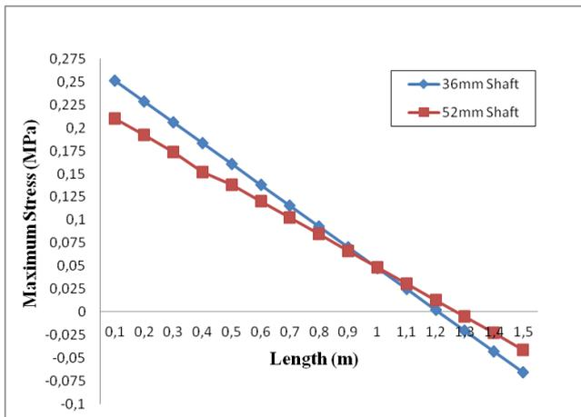
Figure 24. 1st Model-Length-Maximum stress
