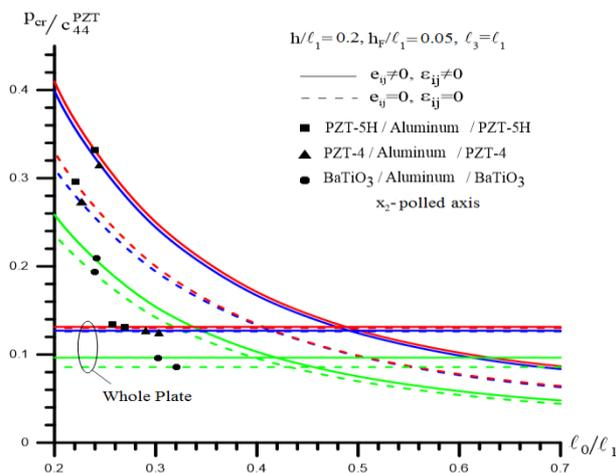
**Figure 3.** The critical buckling delamination force values of the PZT/Aluminum/PZT sandwich rectangular thick plate for the different PZT materials and  $\ell_0$  crack lengths
