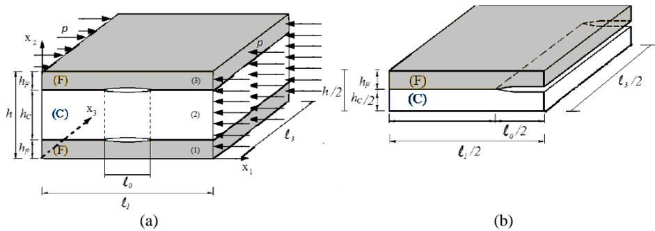
**Figure 1.** The geometry of the plate and the considered external forces; solution domain (a), one-eighth of the region (b)
