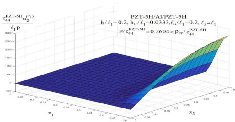
**Figure 2.** The surface graph of the PZT-5H/Aluminum/PZT-5H sandwich rectangular thick plate for  $p/c_{44}^{PZT-5H} = 0.2604$  in the section  $x_2 = h_F + h_C + 0^+$
