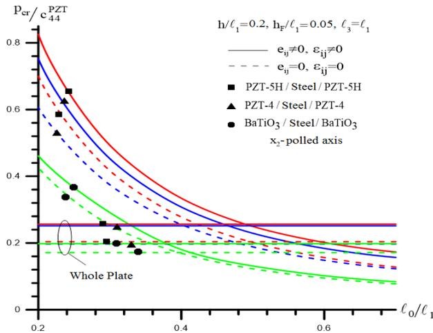
**Figure 4.** The critical buckling delamination force values of the PZT/Steel/PZT sandwich rectangular thick plate for the different PZT materials and  $l_0$  crack lengths
