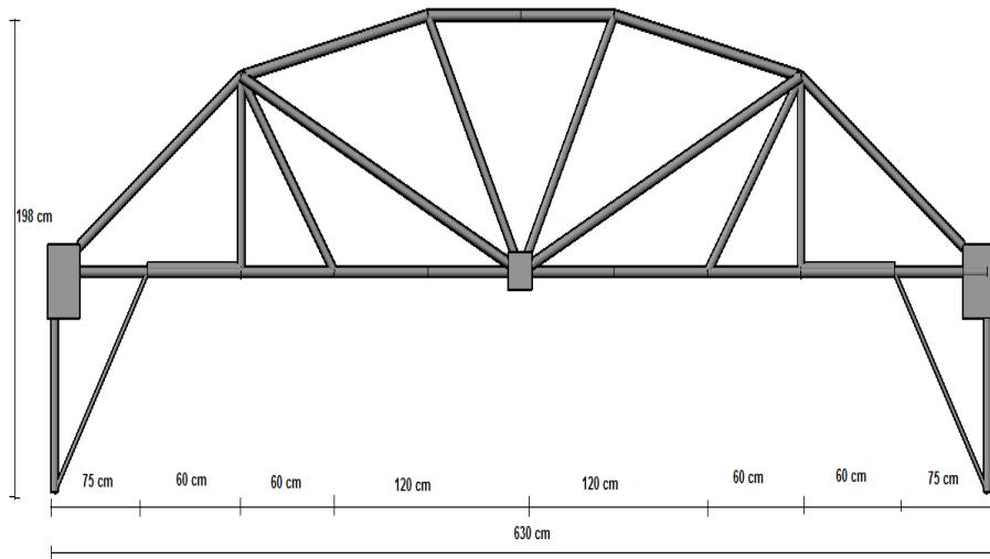
**Figure 1.** Front view of steel bridge designed in AutoCAD program
