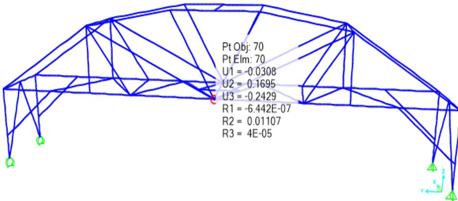
Figure 6. Displacement values in FE model
