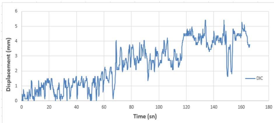
**Figure 4.** Displacement of reference point marked in the steel bridge
