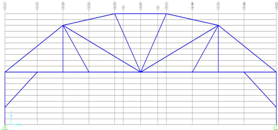
Figure 5. FE model of the steel bridge
