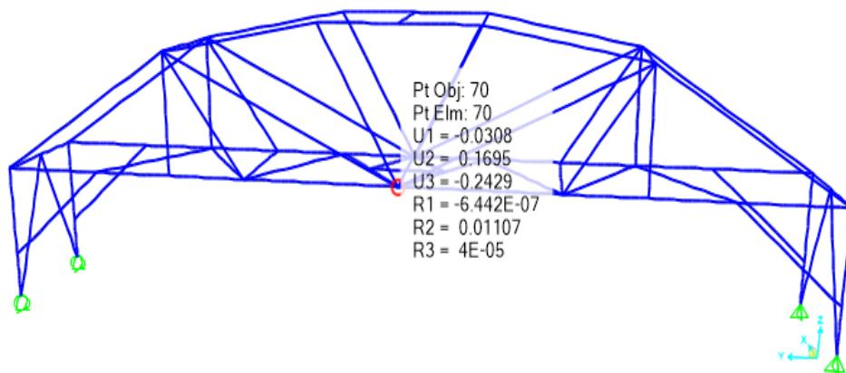
Figure 6. Displacement values in FE model
