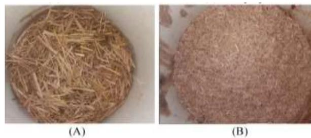
Fig. 1. Prepared stabilizers; (A) straw, (B) rice husk
