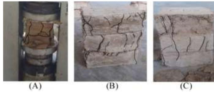
Fig. 4. Failure pattern under compressive loads
