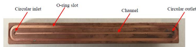
Figure 4. Photograph of a test section [18].
