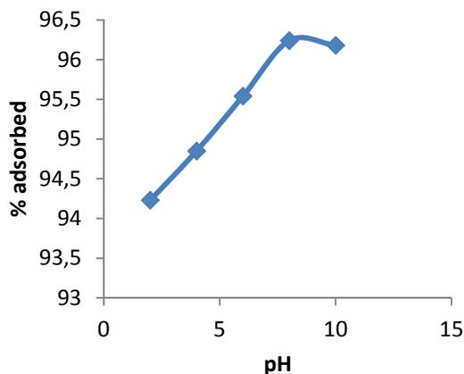
**Figure 1.** Effect of pH on adsorption of CV by KPAC
