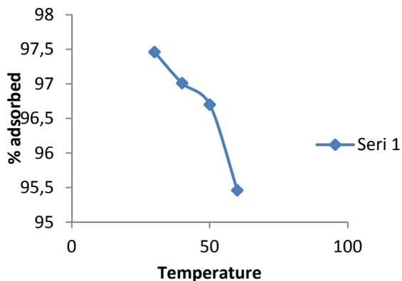
Figure 5. Effect of temperature on adsorption of CV by KPAC.
