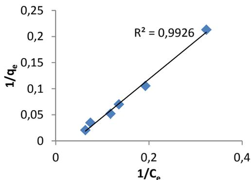
**Figure 7a.** Langmuir Isotherm plot of CV adsorption by KPAC
