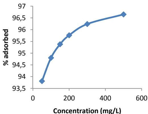
**Figure 2.** Effect of initial concentration on adsorption of CV by KPAC
