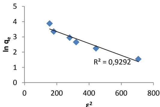
Figure 7c. Dubinin-Radushkevich Isotherm plot of CV adsorption by KPAC
