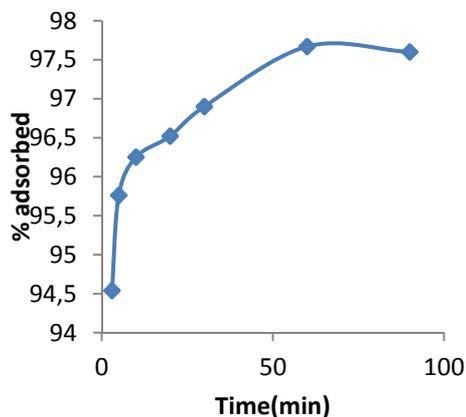
Figure 3. Effect of contact time on adsorption of CV by KPAC
