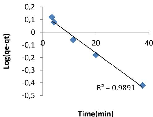
**Figure 6a.** Pseudo first order kinetic plot of CV adsorption by KPAC.
