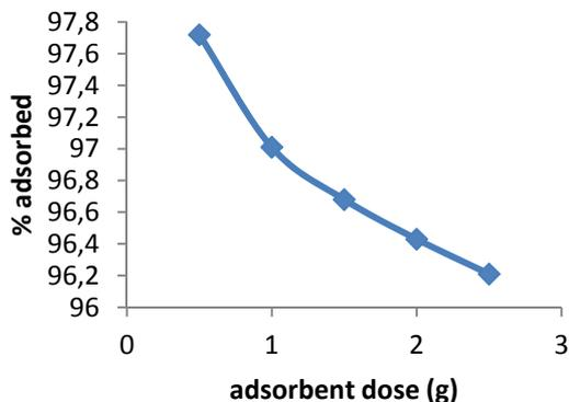
Figure 4. Effect of dosage on adsorption of CV by KPAC
